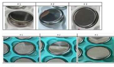
Failure example of leaking in reliability test
