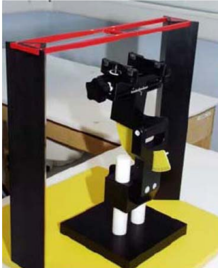
Figure 7 T-coil Phantom & Device Holder
