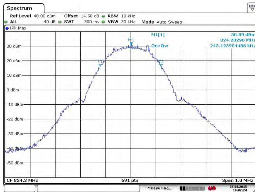
99% Occupied Bandwidth Plot on Channel 128 (824.2 MHz)
