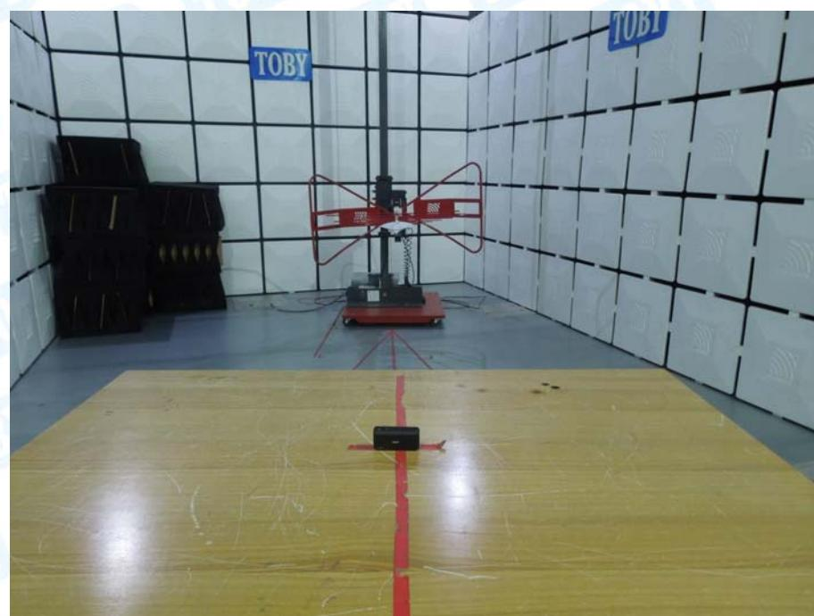
**Photo of Setup for Conducted Emission**
