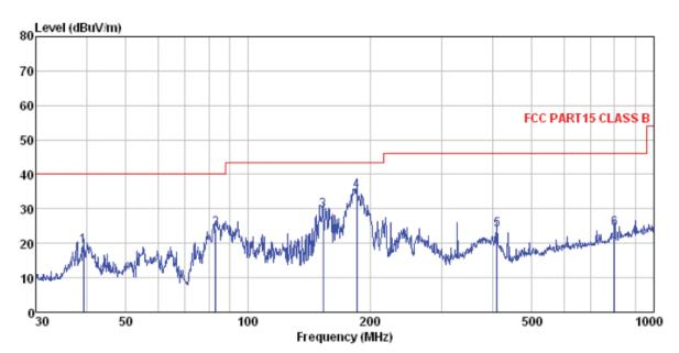
3m chamber FCC PART15 CLASS B 3m VULB9163-2013M HORIZONTAL
