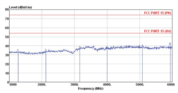
Site Condition : 3m chamber : FCC PART 15 (PK) 3m BBHA9120D ANT(>1GHZ) HORIZONTAL
