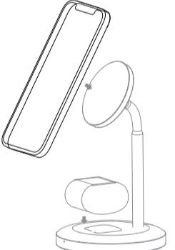
When the wireless charger is connected to an ordinary 5V adapter through Type-C to Type-C cable (Standard cable for this product) or USB-A to USB-C cable, the product works in ordinary wireless charging mode and only supports single 5W load. If you use QC, PD standard adapter, the product will work in quick wireless charging mode and supports 7.5W/10W/15W load.
