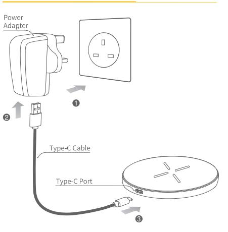
① Connect the power adapter to socket.
