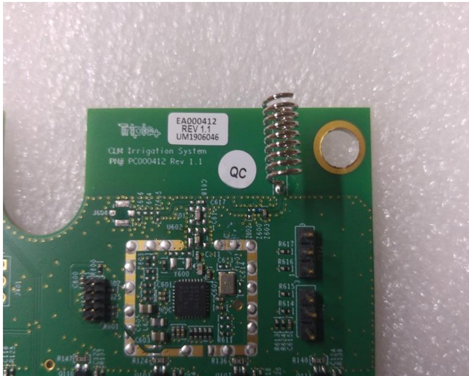
Photograph No.4 Irrigation Controller unit antenna
