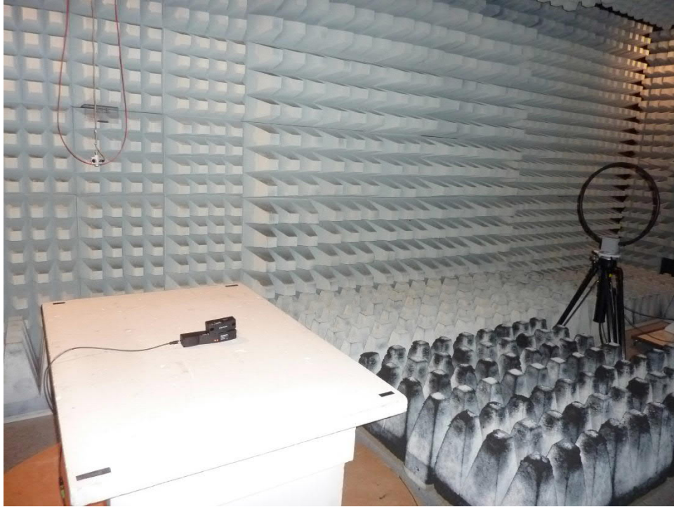
191513AS_01: Preliminary measurement H-Field 9 kHz – 30 MHz
