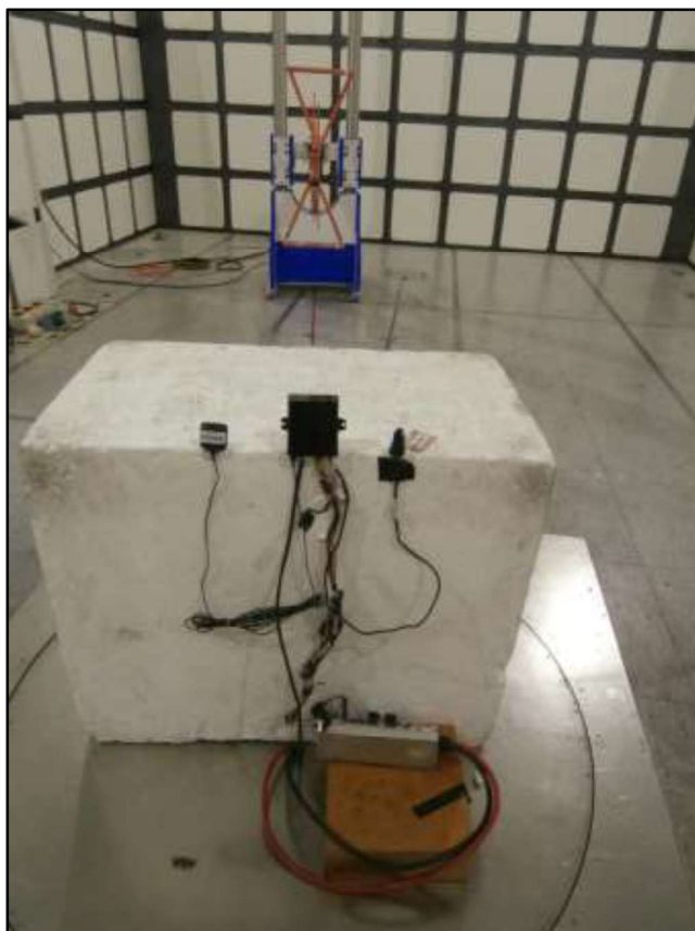
Figure 63 - Test Setup - 30 MHz to 1 GHz – Y Orientation
