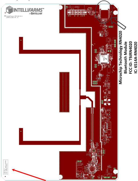
FCC and Industry Canada identifiers screened on PCB. Additional module label use and placement information included in OEM installation Manual
