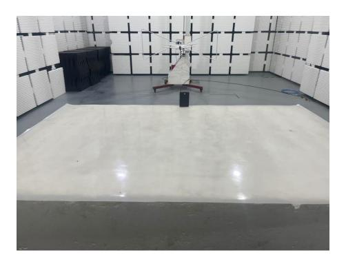
Set-up for Radiated Emission (RE), Above 1GHz
