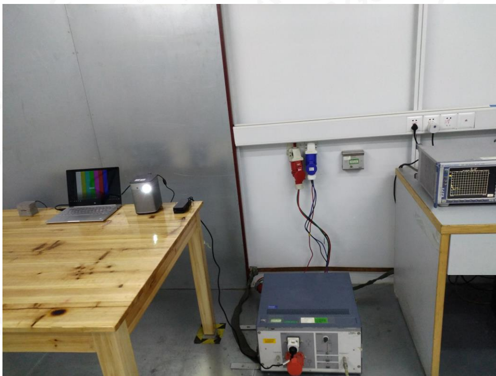
FCC RADIATED EMISSION TEST SETUP BELOW 1GHZ
