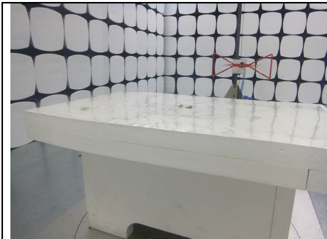
Radiated Spurious Emissions Test Setup Below 1GHz
