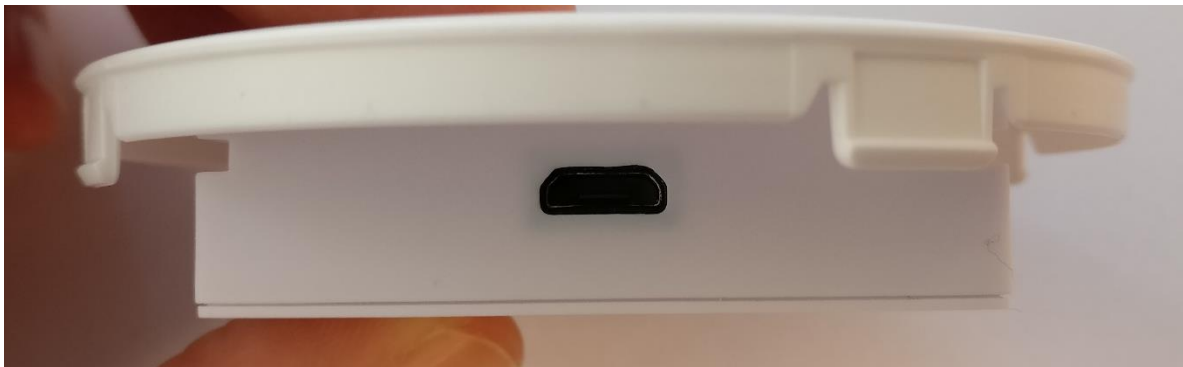
Side view from bottom side with wallmount part removed, showing the uUSB-connector
