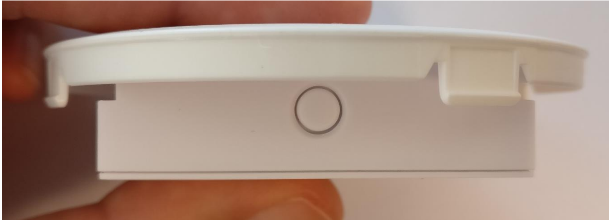
Side view from top side with wallmount part removed, showing the on/off key
