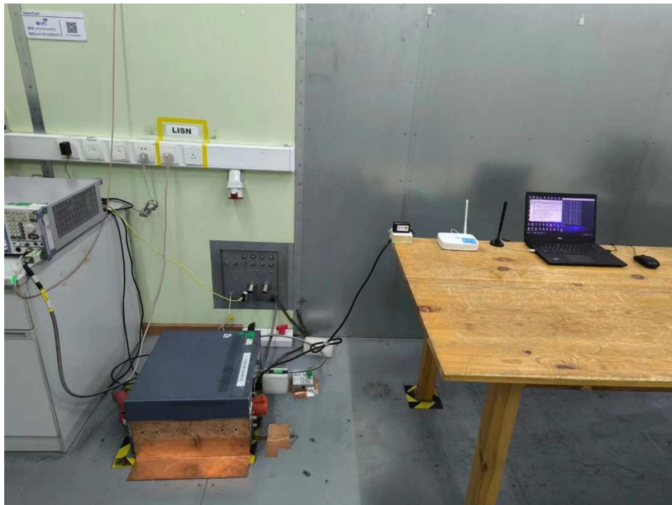
Photograph 3: Set-up for Conducted Emissions, AC Mains
