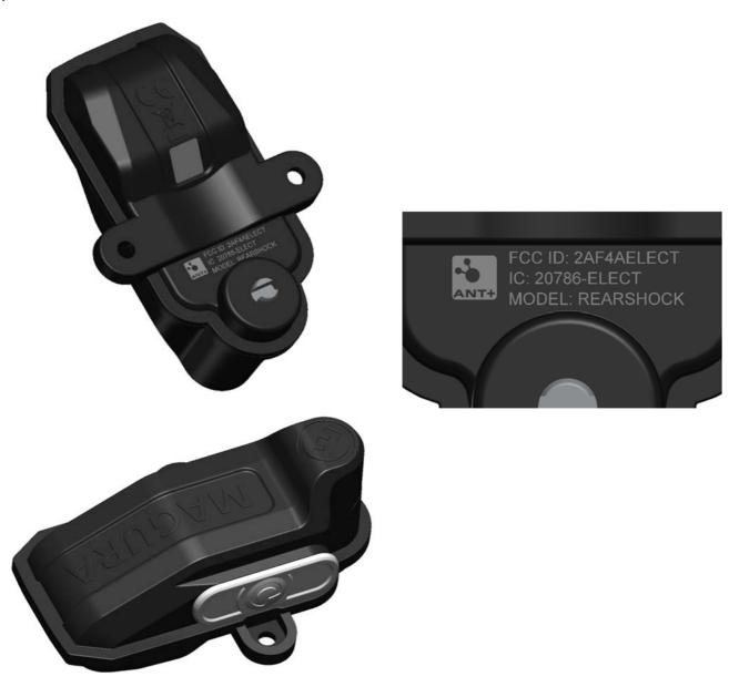
Delivery state: The Module is mounted to the rear shock absorber; at the time of purchase is the label not visible. The label is accessible after removing the two Torx screws.
