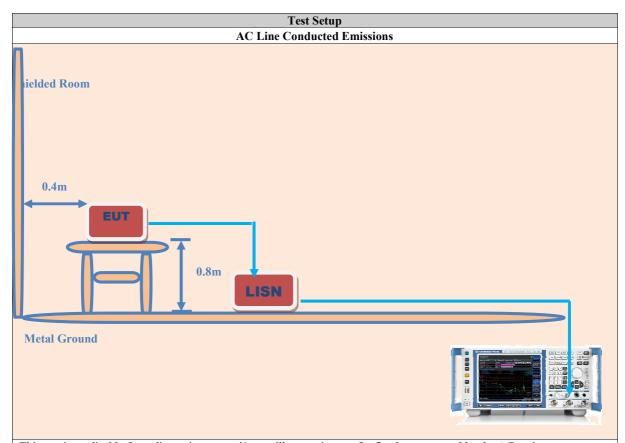
This test is applicable for radio equipment and/or ancillary equipment for fixed use powered by the AC mains. This test shall be performed on a representative configuration of the radio equipment, the associated ancillary equipment, or a representative configuration of the combination of radio and ancillary equipment. This test assesses the level of internally generated electrical noise present on the AC power input/output ports.
