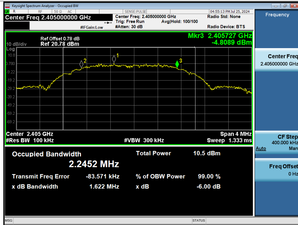
-6dB Bandwidth NVNT Thread 2440MHz Ant1
