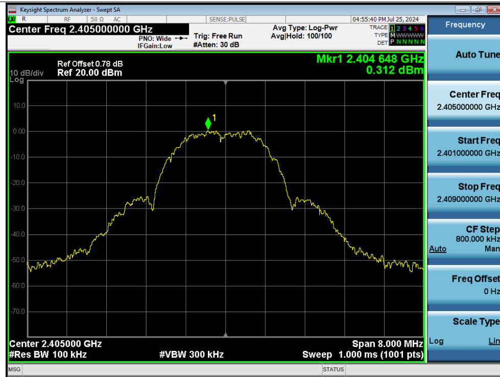
Band Edge NVNT Thread 2405MHz Ant1 Emission
