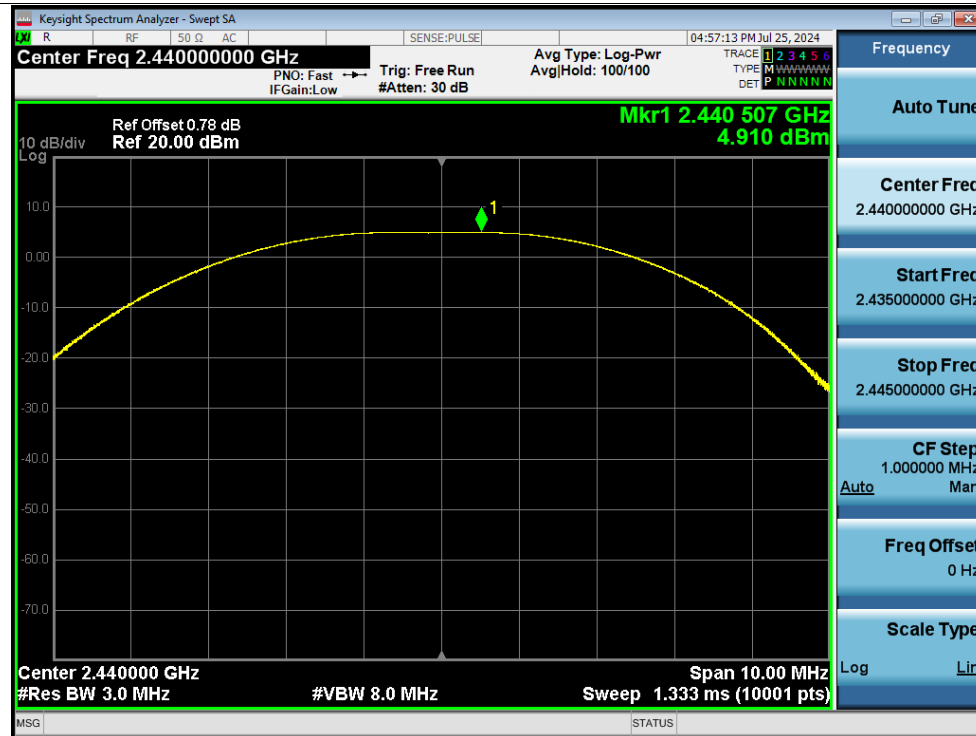
Power NVNT Thread 2440MHz Ant1
