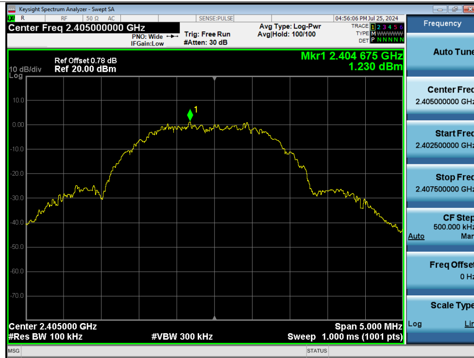
Tx. Spurious NVNT Thread 2405MHz Ant1 Emission
