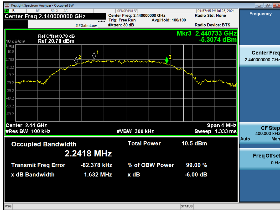
-6dB Bandwidth NVNT Thread 2440MHz Ant1
