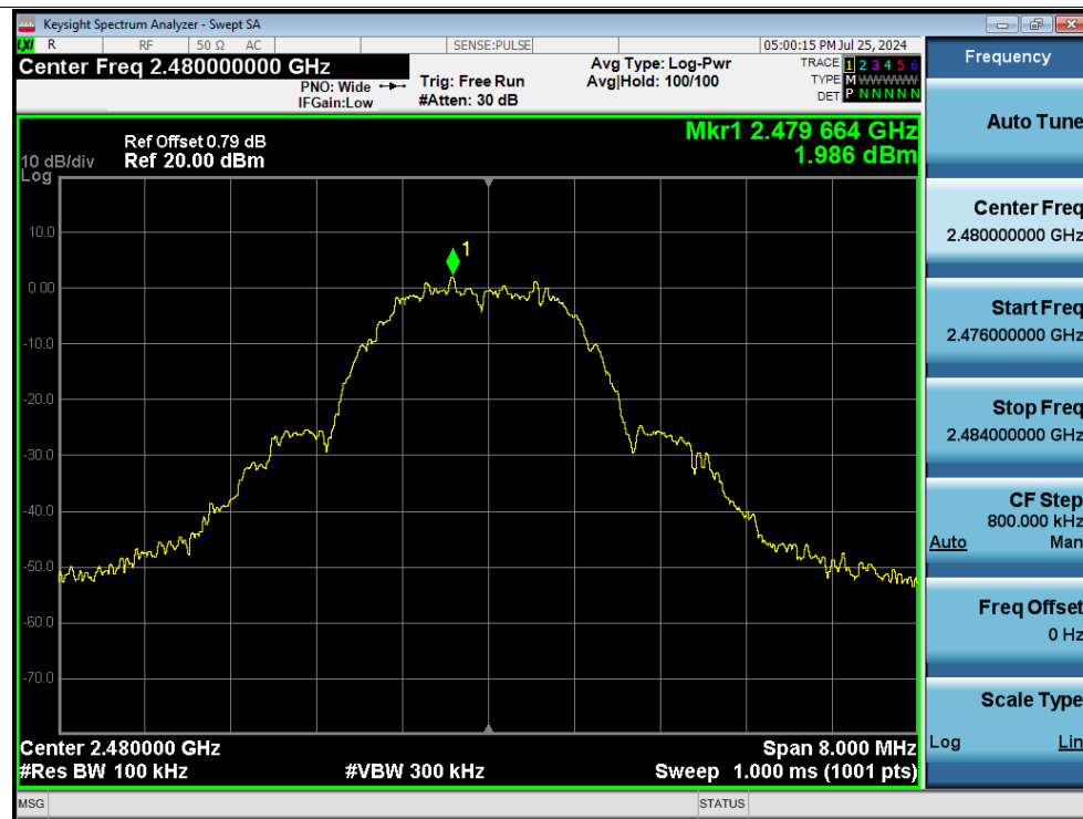
Band Edge NVNT Thread 2480MHz Ant1 Emission
