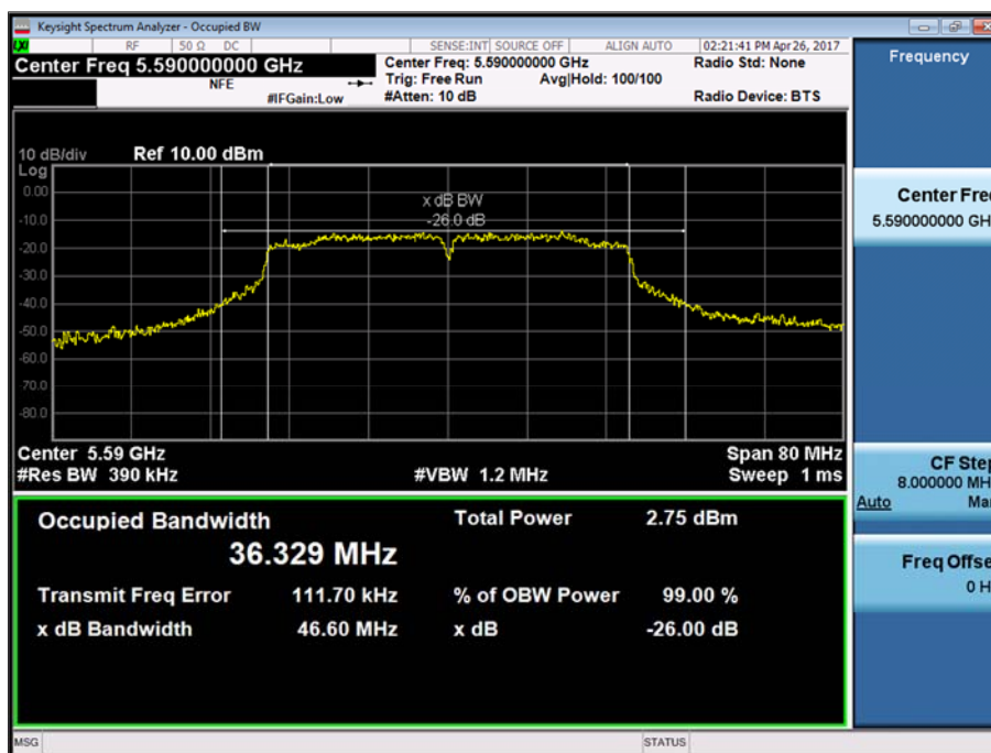
Figure 53 - U-NII 2c - 5590 MHz - 26 dB Bandwidth
