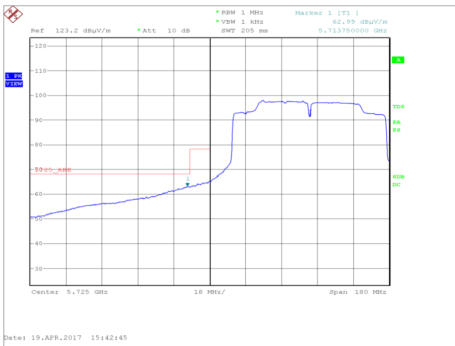
Figure 119 - U-NII 3 - Authorised Band Edge at 5725 MHz - Widest Emission Bandwidth
