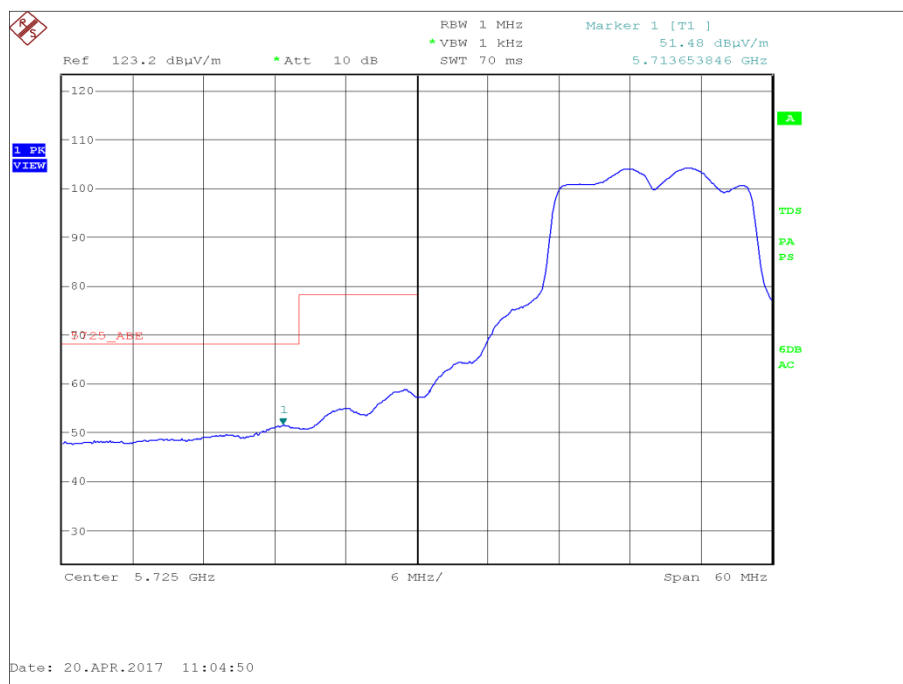
Figure 71 - U-NII 3 - Authorised Band Edge at 5725 MHz - Widest Emission Bandwidth
