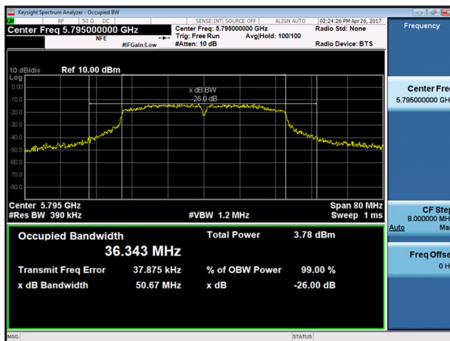
Figure 56 - U-NII 3 - 5795 MHz - 6 dB Bandwidth
