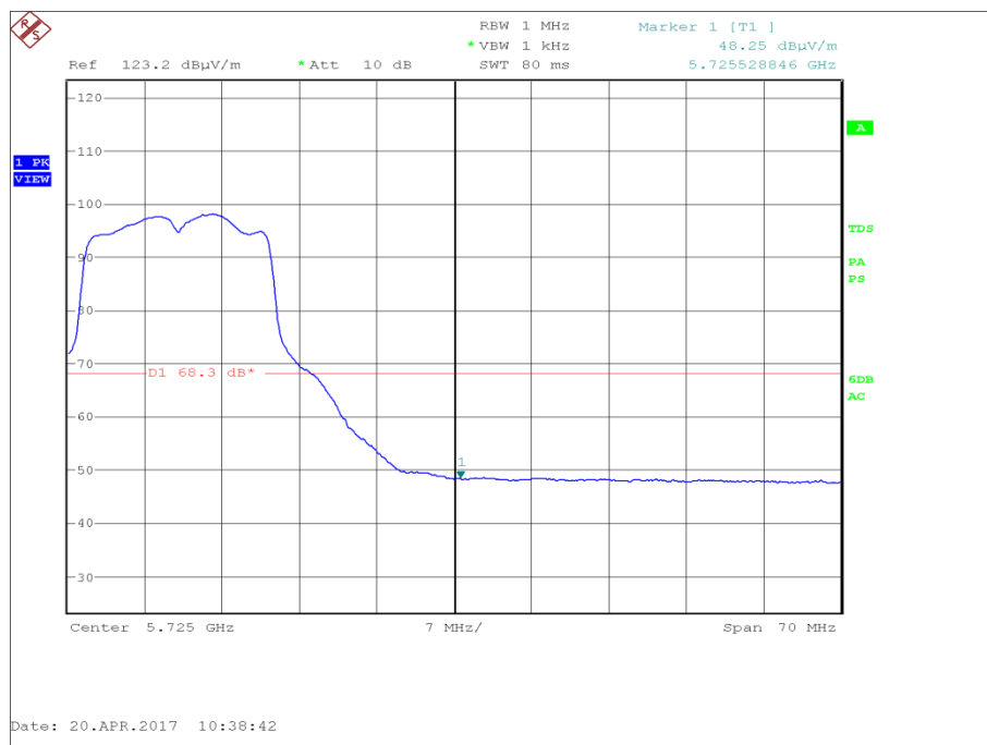
Figure 68 - U-NII 2c - Authorised Band Edge at 5725 MHz - Highest Conducted Power
