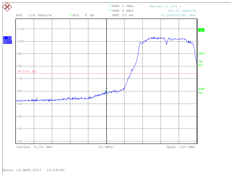
Figure 164 - U-NII 1 - Restricted Band Edge at 5150 MHz - Peak
