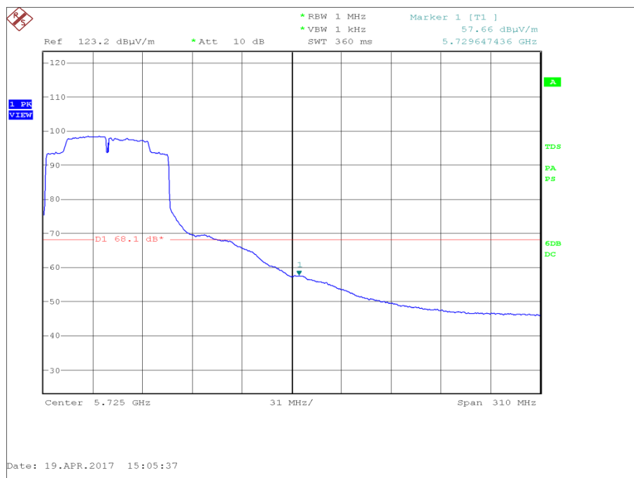
Figure 116 - U-NII 2c - Authorised Band Edge at 5725 MHz - Highest Conducted Power
