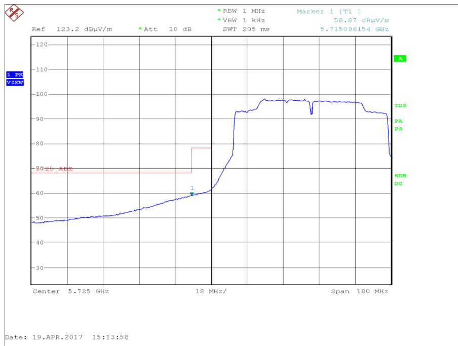
Figure 118 - U-NII 3 - Authorised Band Edge at 5725 MHz - Highest Conducted Power
