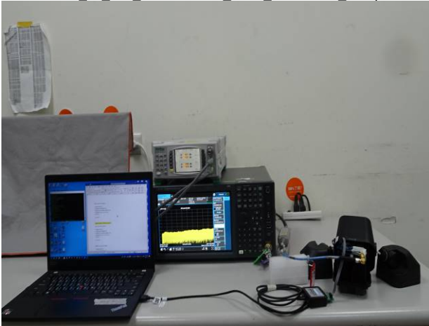
FCC 15 247 902~928MHz LoRa Radiated Setup
