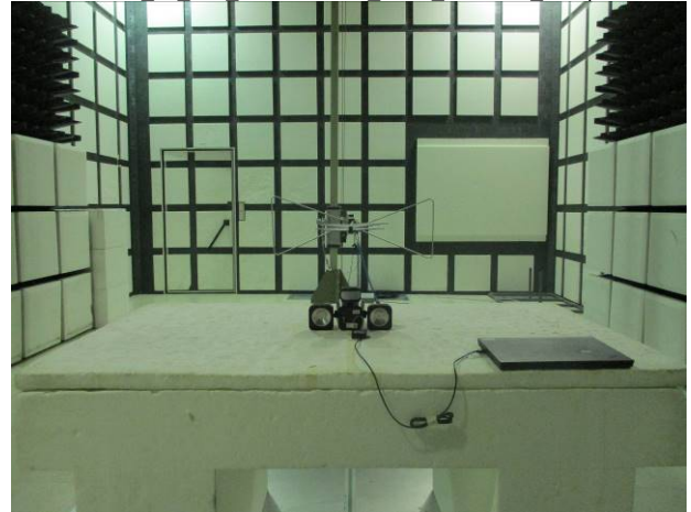
FCC 15 247 902~928MHz LoRa Radiated Setup
