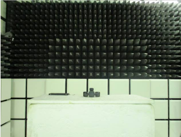
FCC 15 247 902~928MHz LoRa Radiated Setup
