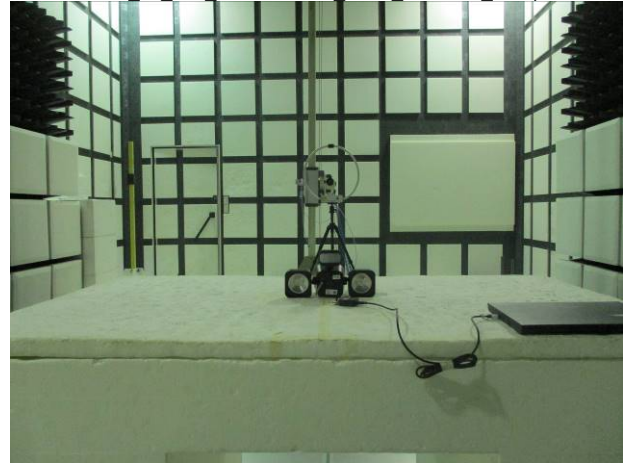
FCC 15 247 902~928MHz LoRa Radiated Setup
