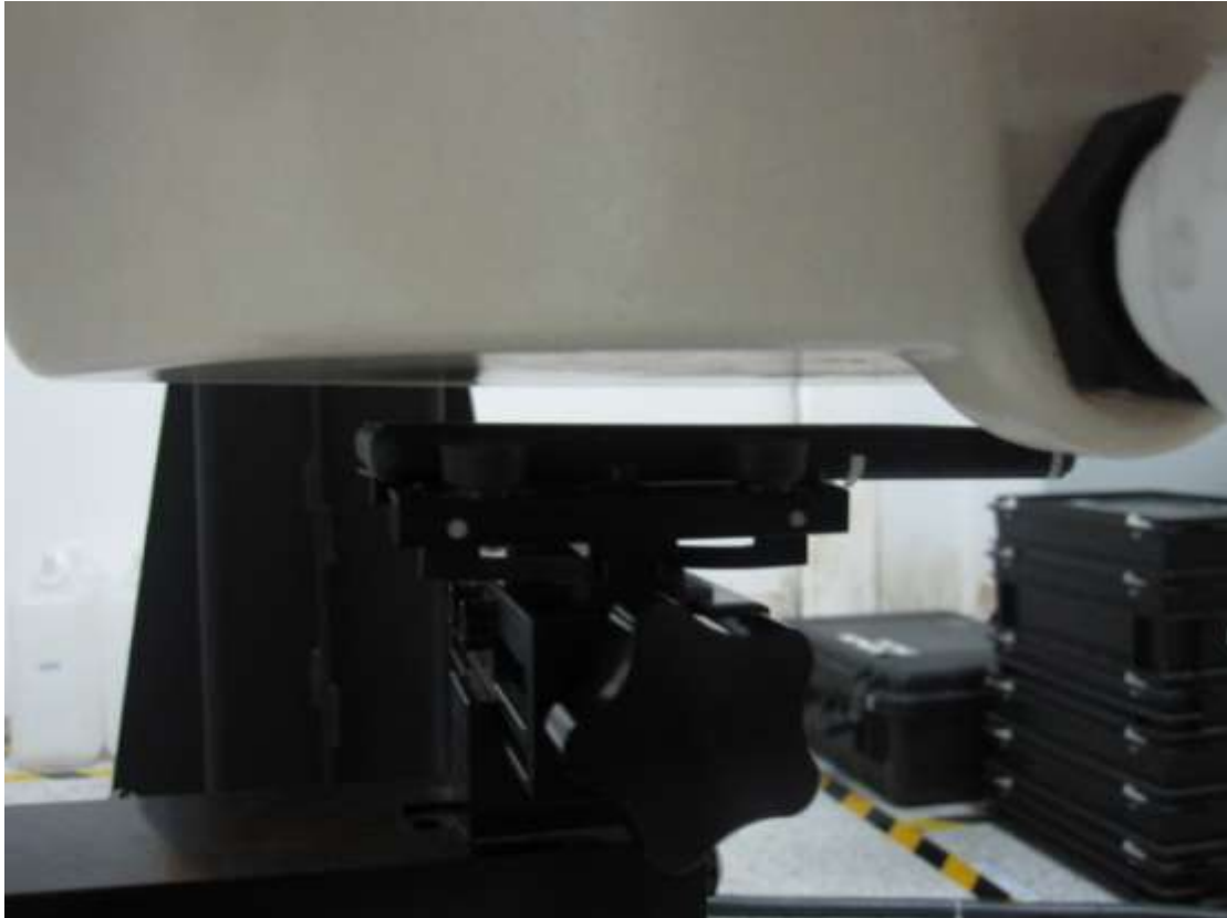
POSITION OF BODY TOWARDS GROUND WITH 10mm DISTANCE
