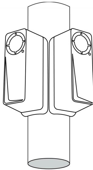
The main thing to consider when choosing the installation method is to ensure a clear view of the detection beam towards the observed area.
