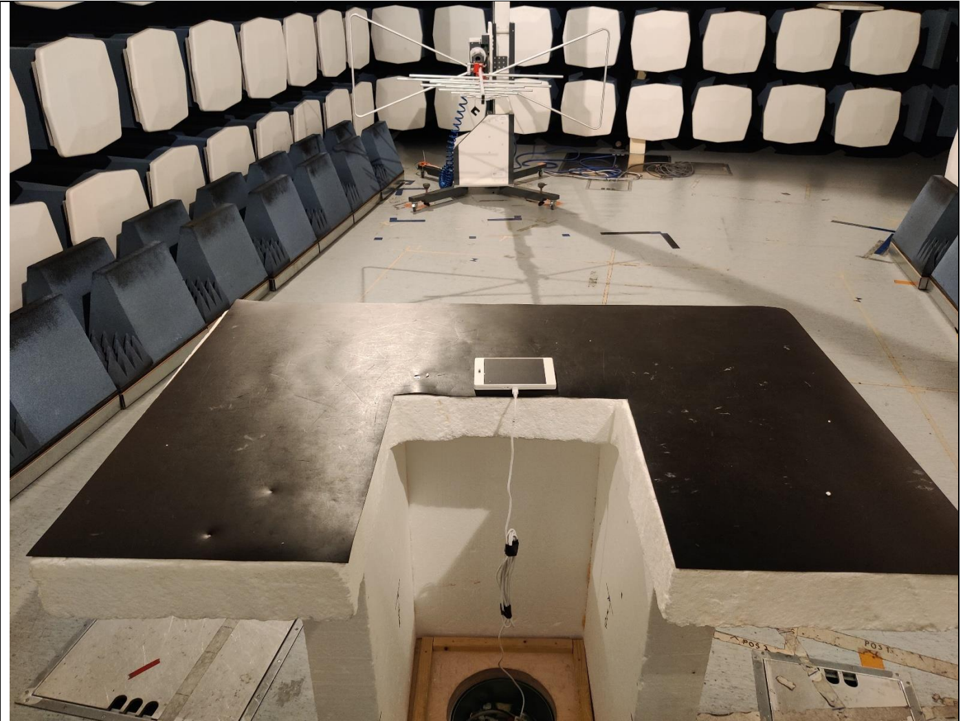
Picture 14, Radiated Spurious Emissions, EUT setup, TX and RX 30 – 1000 MHz
