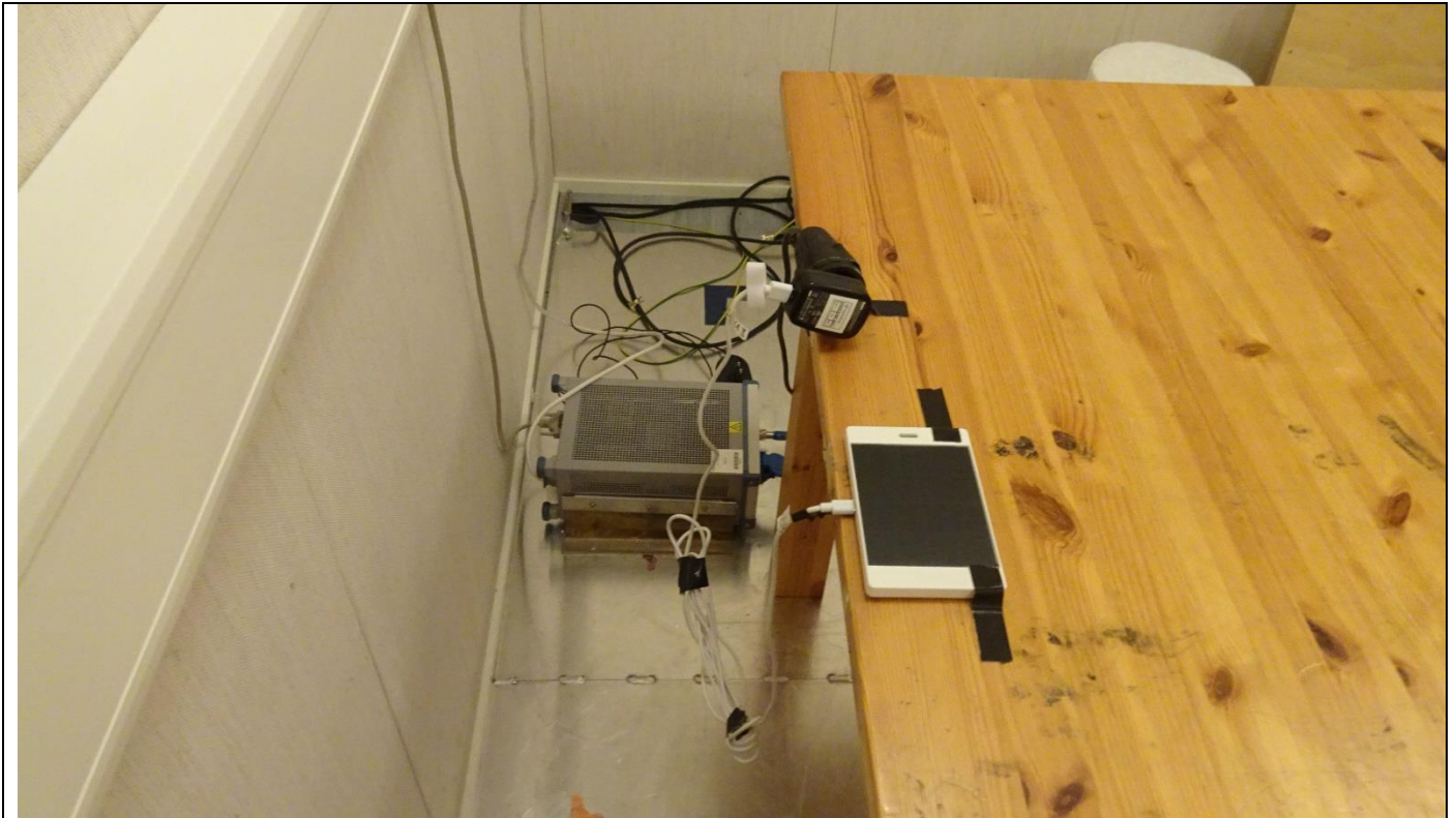
Picture 10, AC Power Line Conducted Emissions
