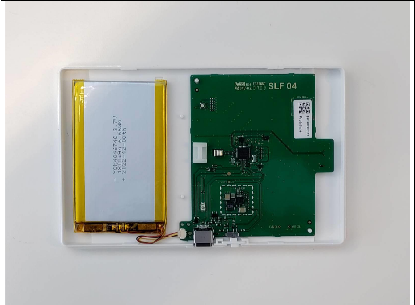
Picture 7, EUT PCB and battery inside B cover
