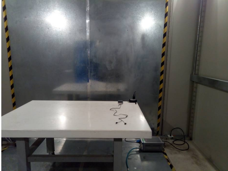
Conducted Emissions - Front View
