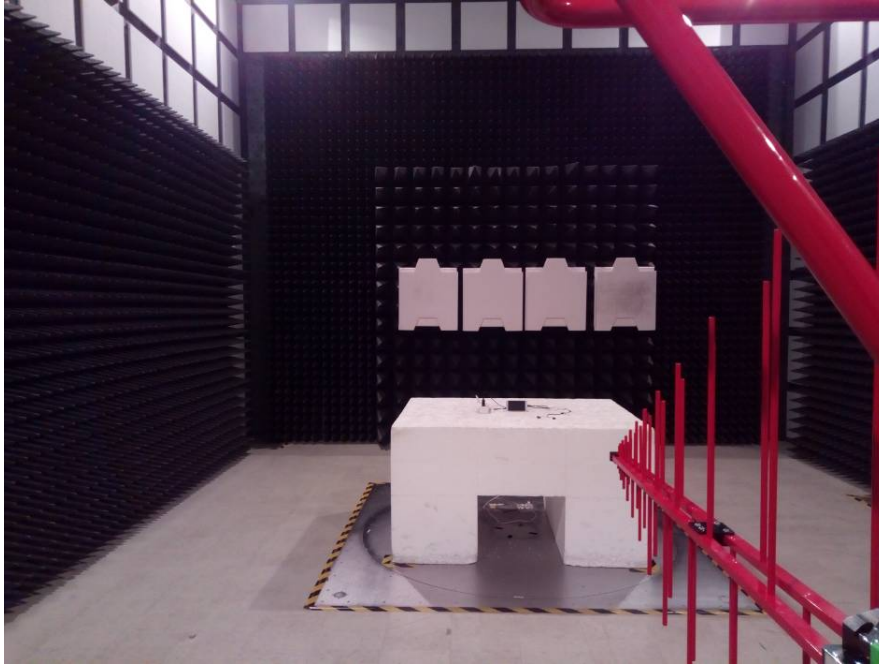
Radiated Emissions View (Below 1 GHz)
