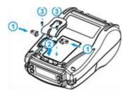
1) Put the left belt clip cradle into the groove, refer to ① in figure above.
