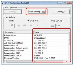
2. Click "on" to set communication mode, such as infrastructure mode. Other information setup: remark: The printer is regarded as terminal device connected with router when the status is infrastructure mode.
