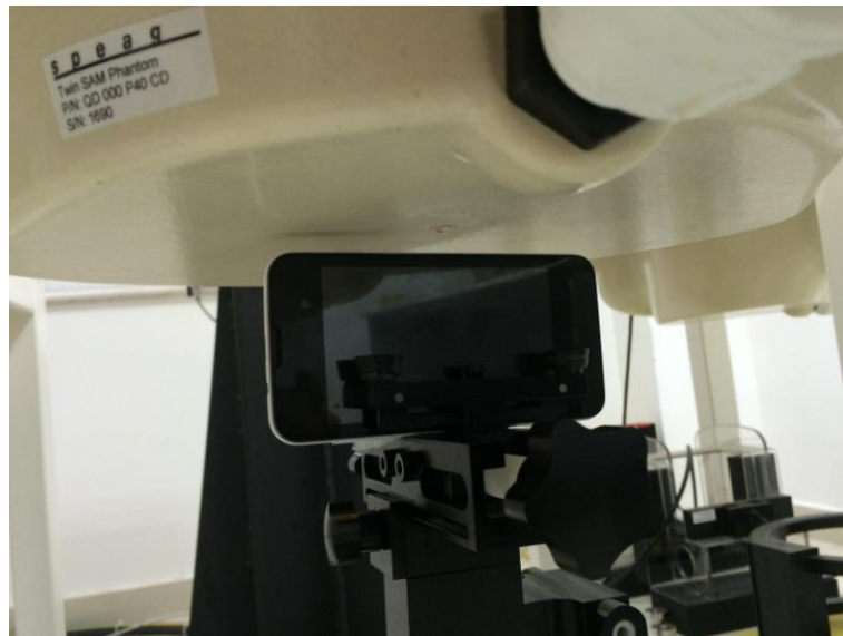
10mm Body-worn Right Side Setup Photo
