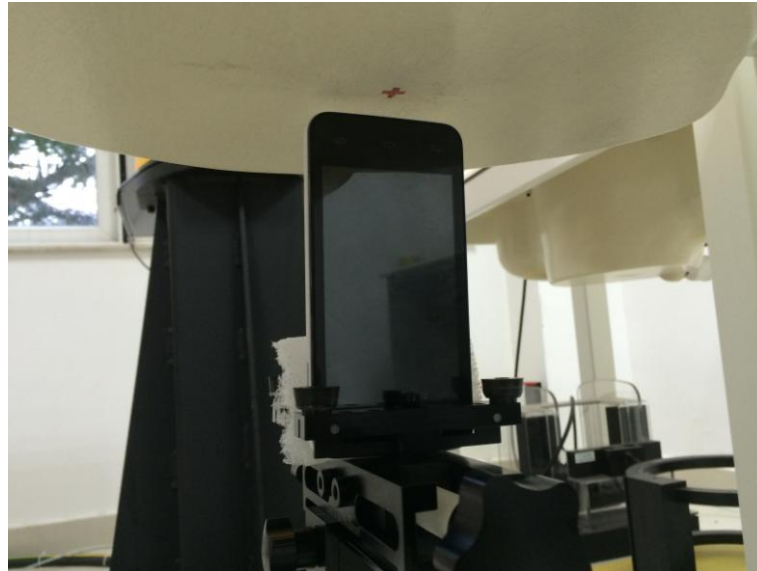
10mm Body-worn Bottom Side Setup Photo
