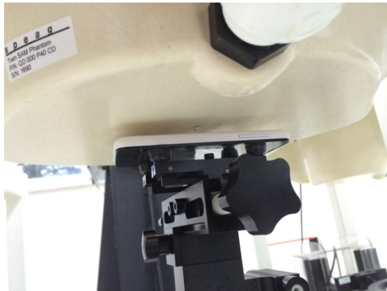
10mm Body-worn Rear Side Setup Photo
