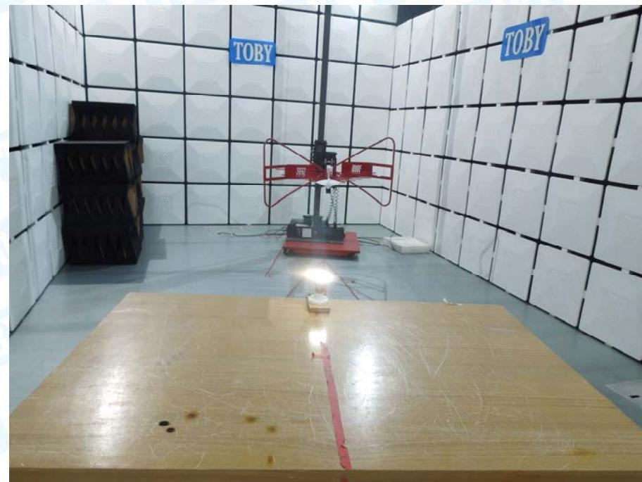
**Photo of Setup for Conducted Emission**
