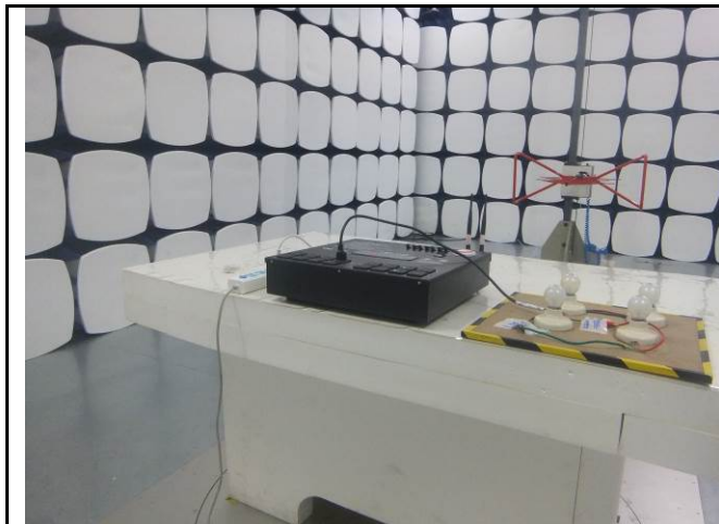
Radiated Spurious Emissions Test Setup Below 1GHz
