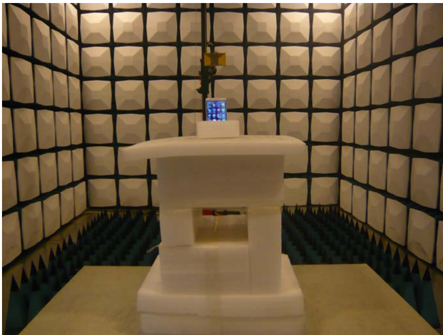
Radiated Emission View (Above 1GHz)
