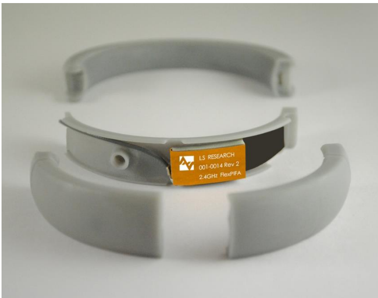
Figure 28: FlexPIFA integrated into bracelet
