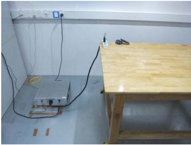
Conducted Emissions Test Setup – Front View
