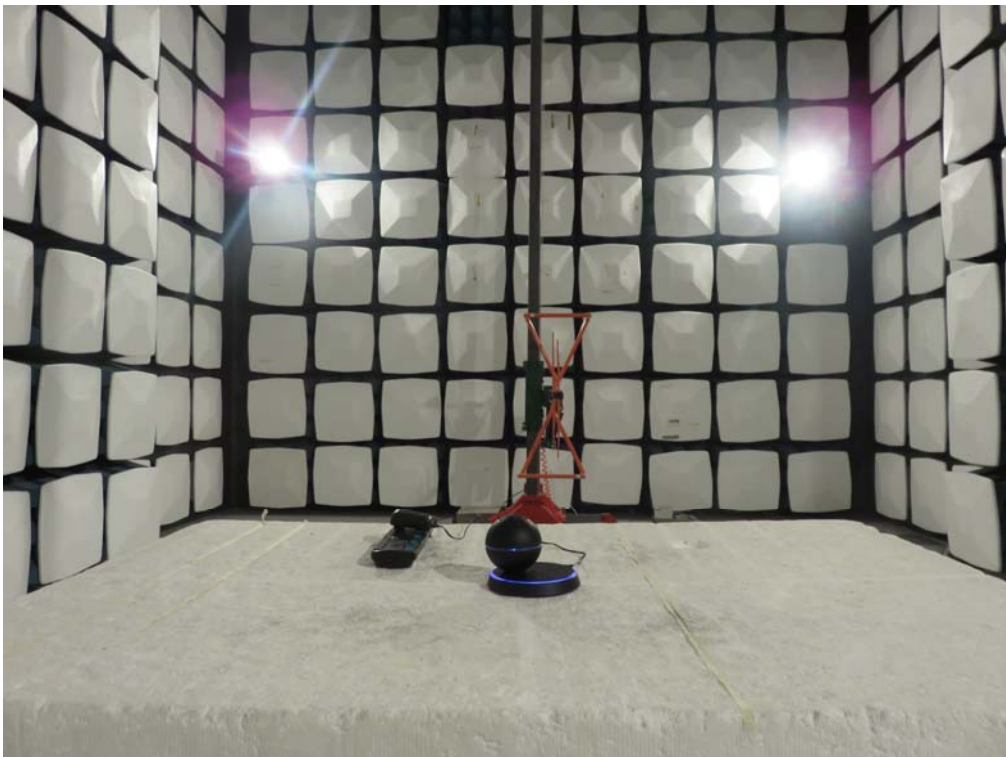
FCC RADIATED EMISSION TEST SETUP
