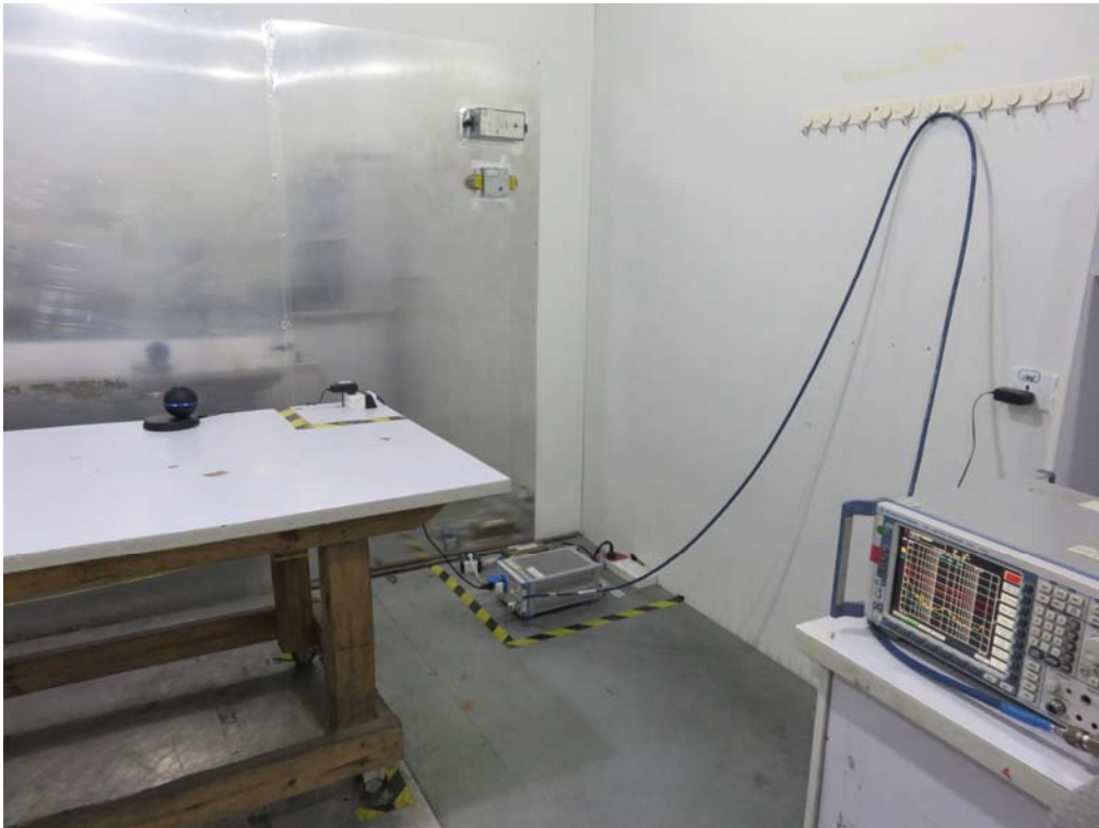
FCC RADIATED EMISSION TEST SETUP
