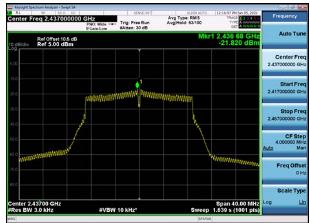
Power spectral density-802.11n(HT20) ,2437MHz
