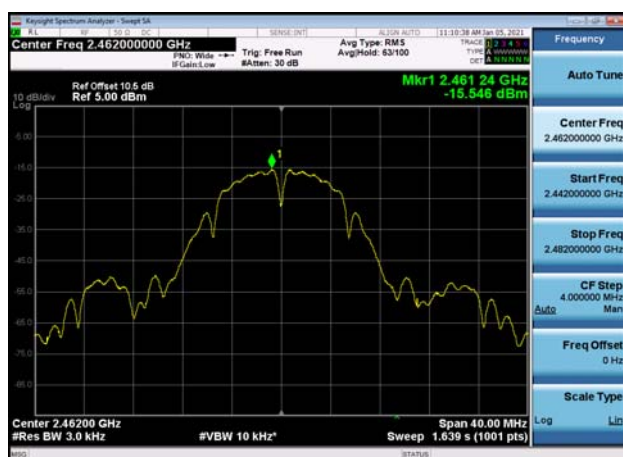
Power spectral density-802.11g ,2437MHz
