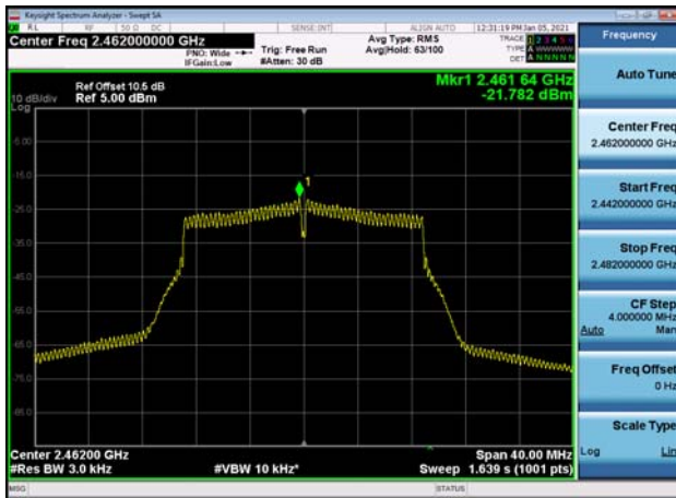
Power spectral density-802.11n(HT20) ,2462MHz
