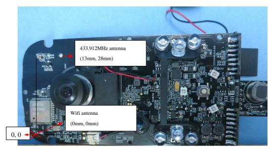
The power densities of up to 2 antennas located within a 90 cm<sup>2</sup> region at 1cm intervals are estimated first. Then the power densities computed for each antenna are summed.
