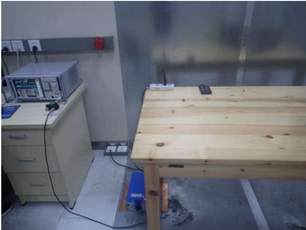
FCC RADIATED EMISSION TEST SETUP
