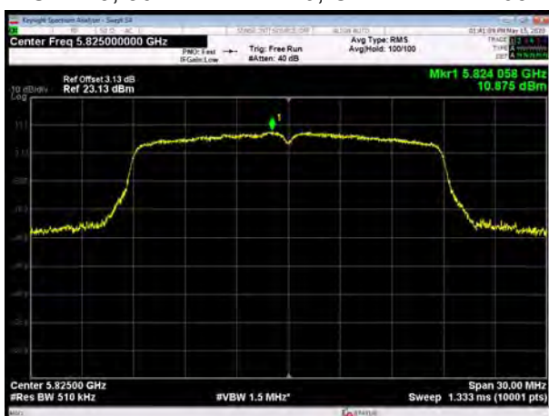
U-NII-3, 802.11ac VHT80, Channel No.: 155
