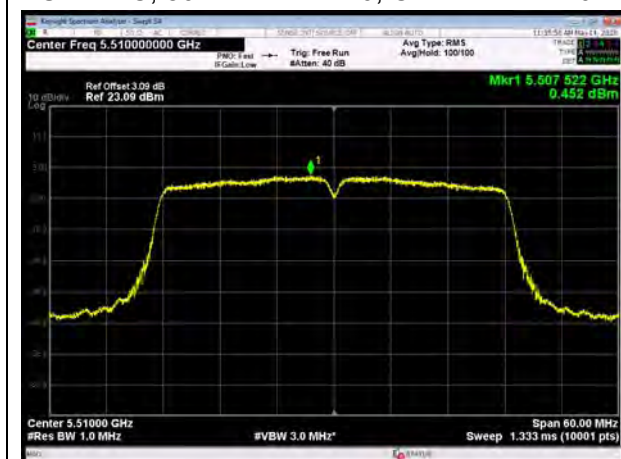
U-NII-2C, 802.11ac VHT40, Channel No.: 110
