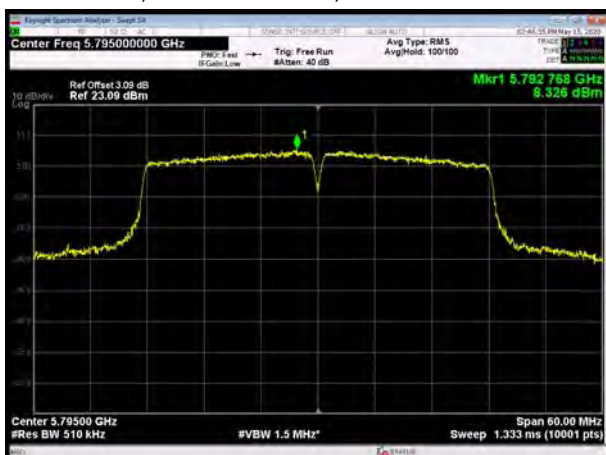
U-NII-3, 802.11ac VHT40, Channel No.: 151
