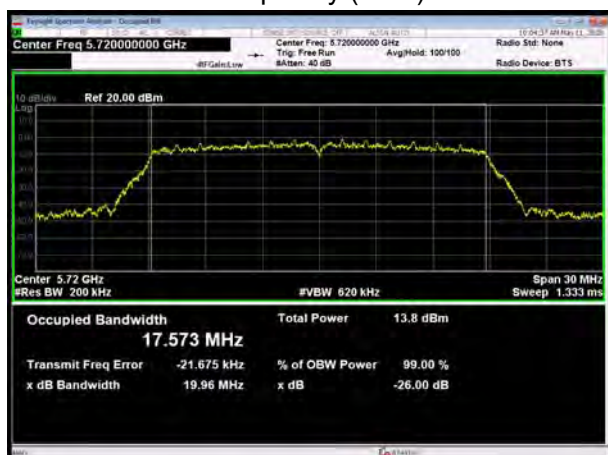
U-NII-2C, 802.11n HT20 Carrier frequency (MHz): 5720
