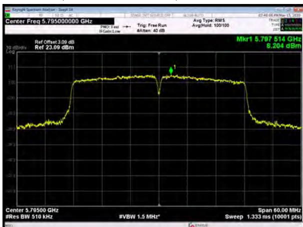
U-NII-3, 802.11ac VHT40, Channel No.: 159
