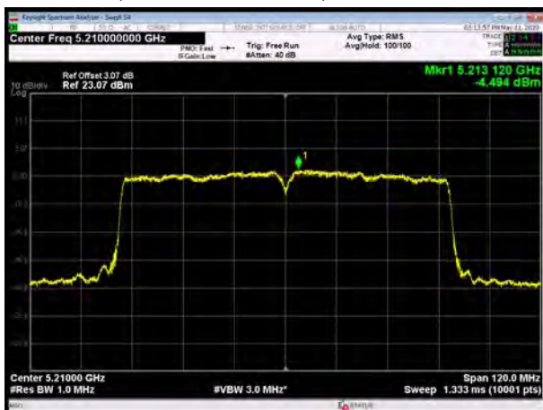
U-NII-1, 802.11ac VHT80, Channel No.: 42
