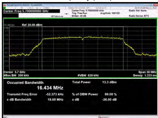
U-NII-2C, 802.11a Carrier frequency (MHz): 5720
