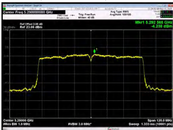
U-NII-2A, 802.11ac VHT80, Channel No.: 58
