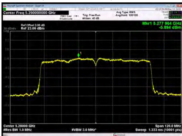
U-NII-2A, 802.11ac VHT80, Channel No.: 58
