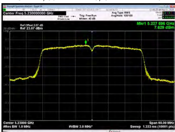
U-NII-1, 802.11ac VHT40, Channel No.: 38
