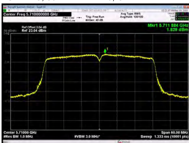
U-NII-2C, 802.11ac VHT80, Channel No.: 138
