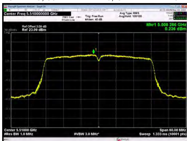
U-NII-2C, 802.11ac VHT40, Channel No.: 110
