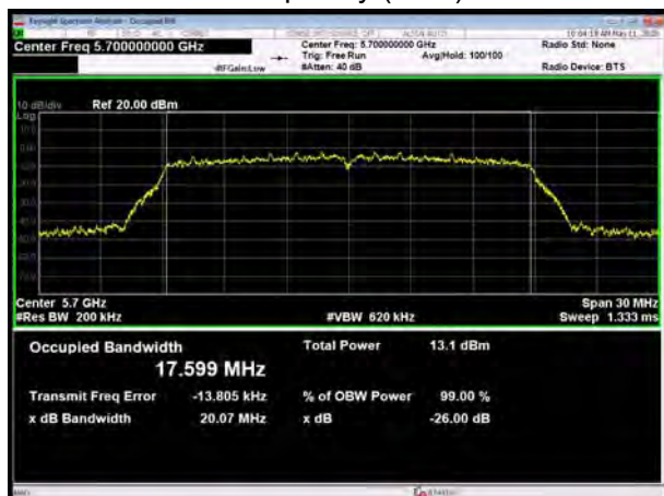
U-NII-2C, 802.11n HT20 Carrier frequency (MHz): 5720
