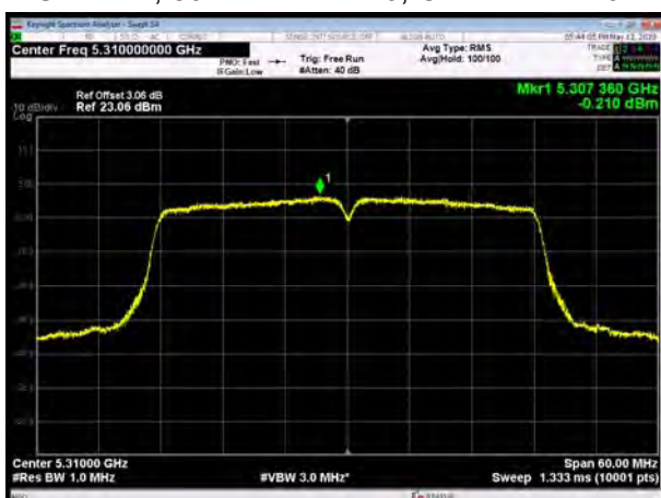
U-NII-2A, 802.11ac VHT40, Channel No.: 62
