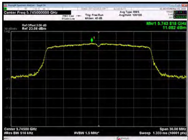
U-NII-3, 802.11ac VHT20, Channel No.: 149
