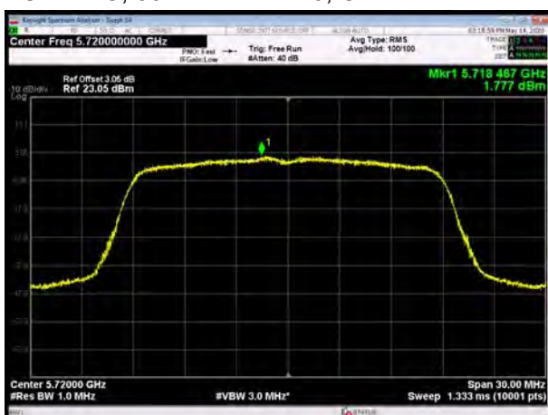
U-NII-2C, 802.11ac VHT80, Channel No.: 106
