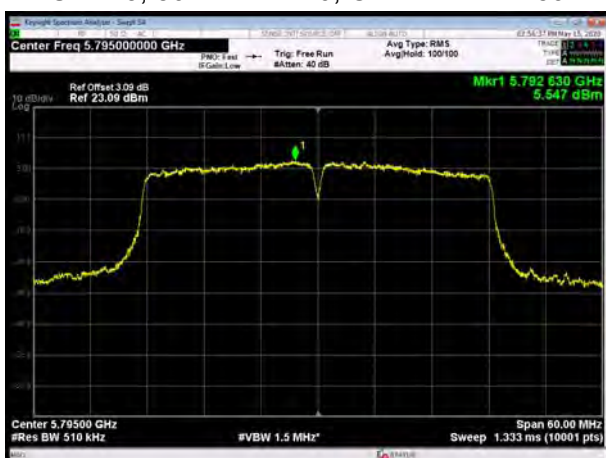
U-NII-3, 802.11ac VHT80, Channel No.: 155
