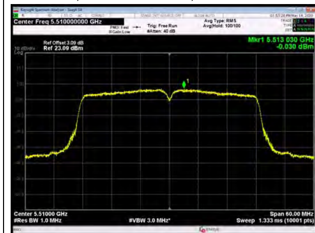
U-NII-2C, 802.11ac VHT40, Channel No.: 110
