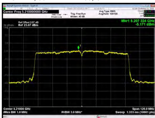
U-NII-1, 802.11ac VHT80, Channel No.: 42
