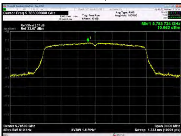
U-NII-3, 802.11ac VHT20, Channel No.: 165
