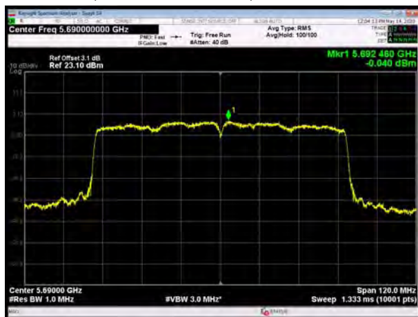
U-NII-2C, 802.11ac VHT80, Channel No.: 138
