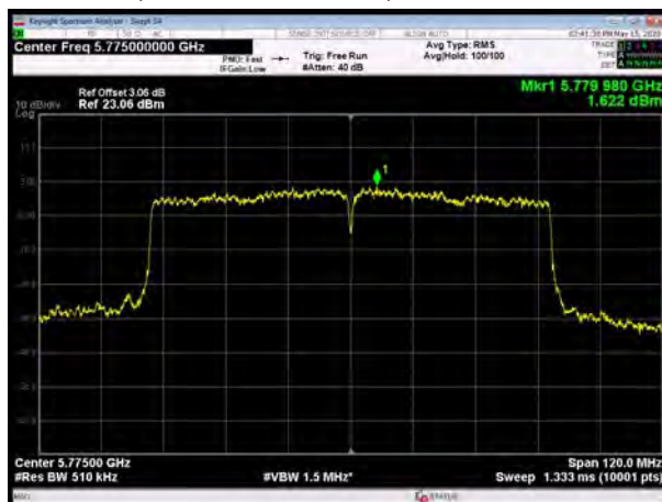
U-NII-3, 802.11ac VHT80, Channel No.: 155
