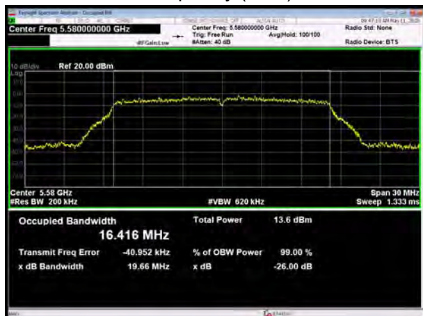
U-NII-2C, 802.11a Carrier frequency (MHz): 5700
