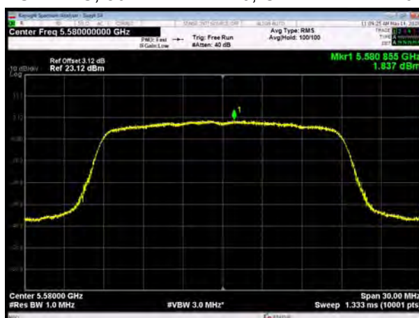
U-NII-2C, 802.11ac VHT20, Channel No.: 140
