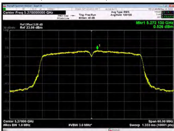
U-NII-2A, 802.11ac VHT40, Channel No.: 62
