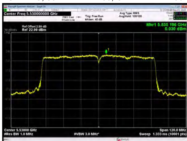
U-NII-2C, 802.11ac VHT80, Channel No.: 138
