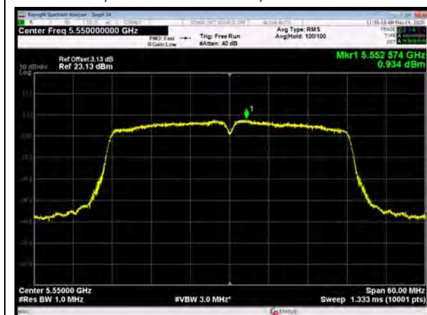
U-NII-2C, 802.11ac VHT40, Channel No.: 110
