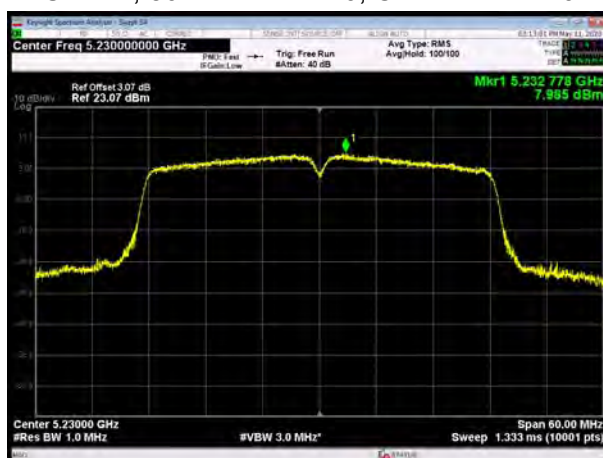
U-NII-1, 802.11ac VHT40, Channel No.: 46
