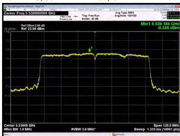
U-NII-2C, 802.11ac VHT80, Channel No.: 138
