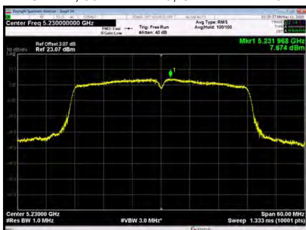
U-NII-1, 802.11ac VHT40, Channel No.: 38
