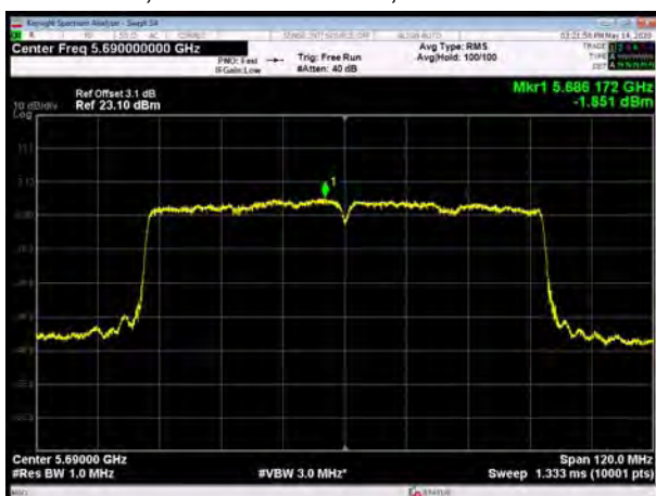
U-NII-2C, 802.11ac VHT80, Channel No.: 138
