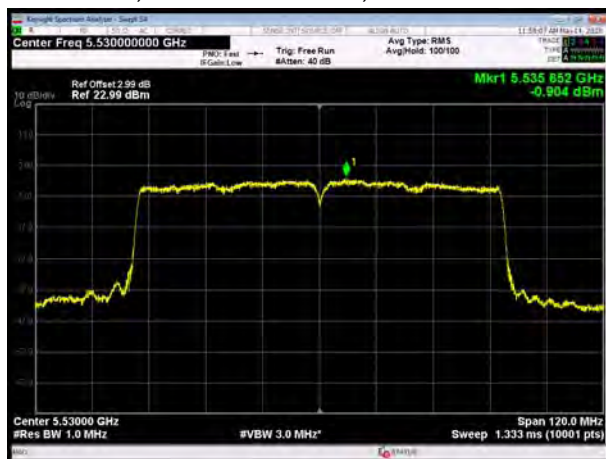
U-NII-2C, 802.11ac VHT80, Channel No.: 138
