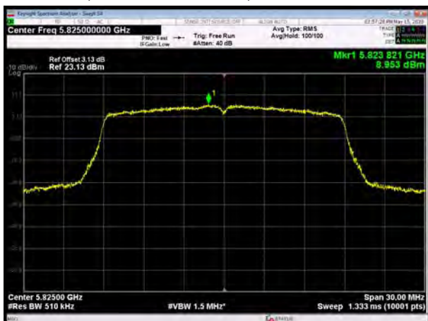
U-NII-3, 802.11ac VHT20, Channel No.: 165
