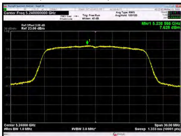
U-NII-1, 802.11ac VHT20, Channel No.: 48
