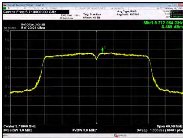
U-NII-2C, 802.11ac VHT40, Channel No.: 142
