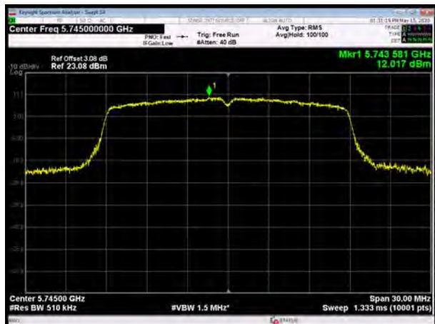
U-NII-3, 802.11ac VHT20, Channel No.: 149
