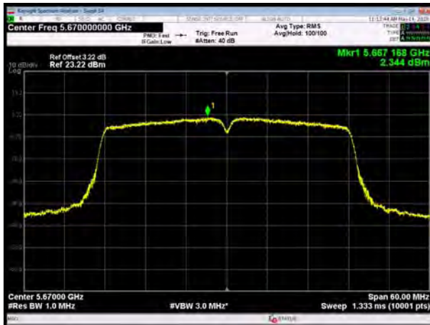
U-NII-2C, 802.11ac VHT40, Channel No.: 142
