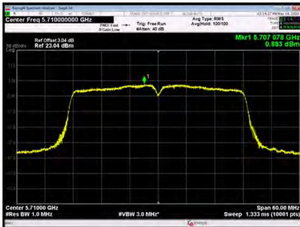
U-NII-2C, 802.11ac VHT40, Channel No.: 142
