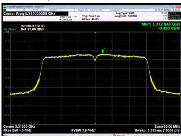
U-NII-2A, 802.11ac VHT80, Channel No.: 58
