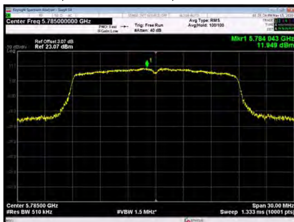
U-NII-3, 802.11ac VHT20, Channel No.: 165
