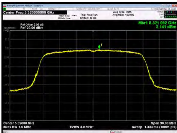
U-NII-2A, 802.11ac VHT20, Channel No.: 64
