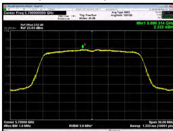
U-NII-2C, 802.11ac VHT20, Channel No.: 140
