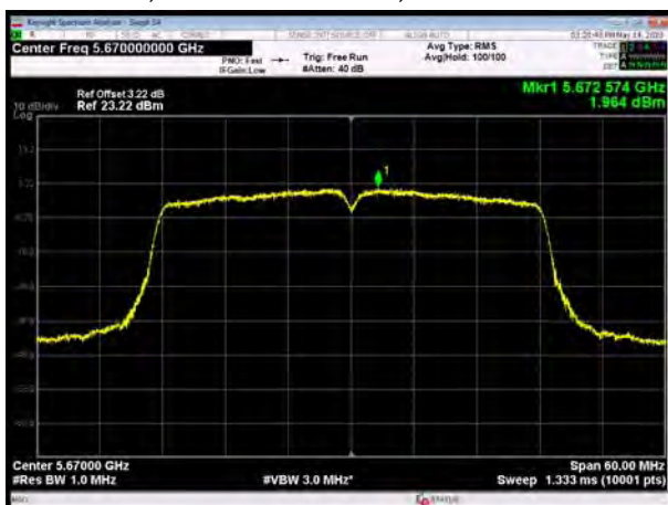
U-NII-2C, 802.11ac VHT40, Channel No.: 142
