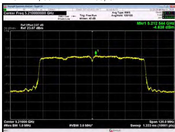
U-NII-1, 802.11ac VHT80, Channel No.: 42
