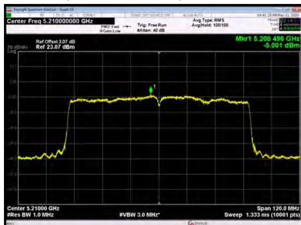
U-NII-1, 802.11ac VHT80, Channel No.: 42
