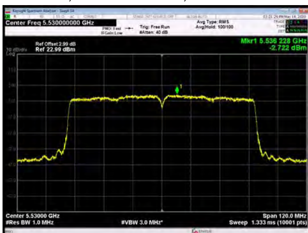
U-NII-2C, 802.11ac VHT80, Channel No.: 106
