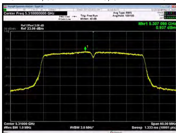
U-NII-2A, 802.11ac VHT40, Channel No.: 62
