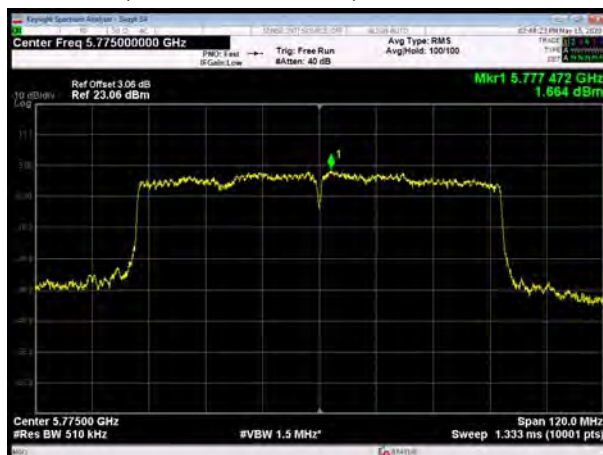
U-NII-3, 802.11ac VHT80, Channel No.: 155
