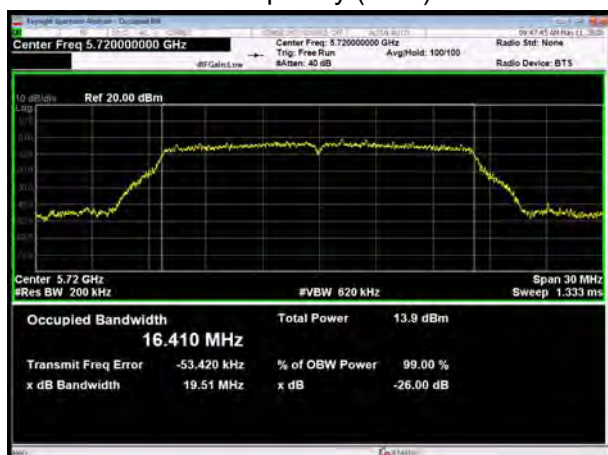
U-NII-2C, 802.11a Carrier frequency (MHz): 5720
