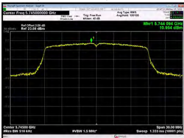
U-NII-3, 802.11ac VHT20, Channel No.: 149
