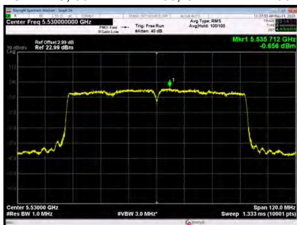
U-NII-2C, 802.11ac VHT80, Channel No.: 138
