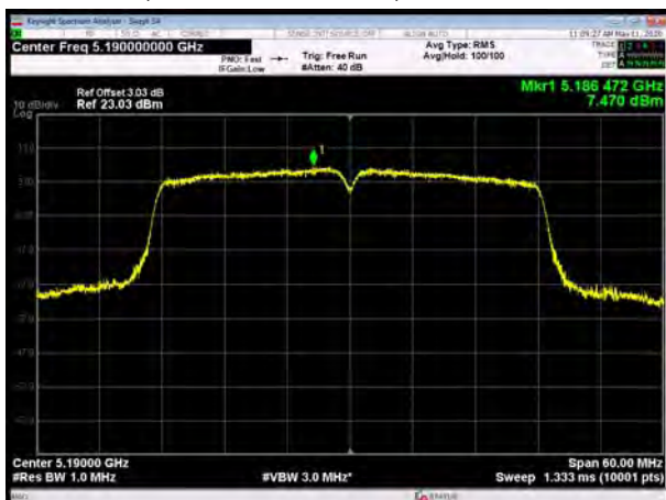
U-NII-1, 802.11ac VHT40, Channel No.: 38
