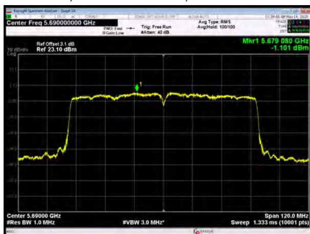
U-NII-2C, 802.11ac VHT80, Channel No.: 138
