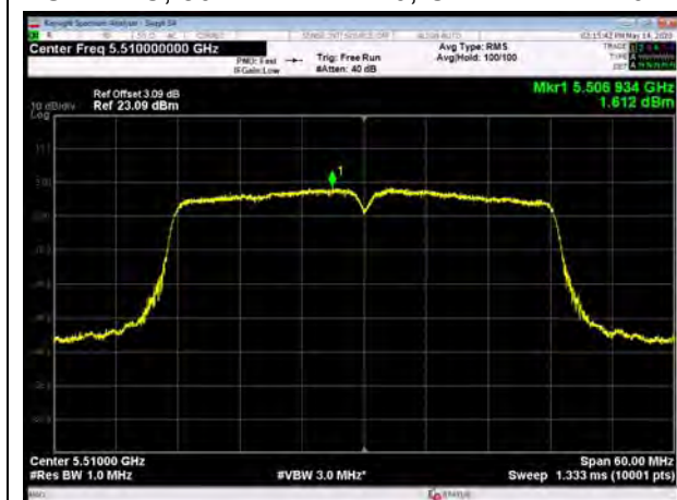
U-NII-2C, 802.11ac VHT40, Channel No.: 110
