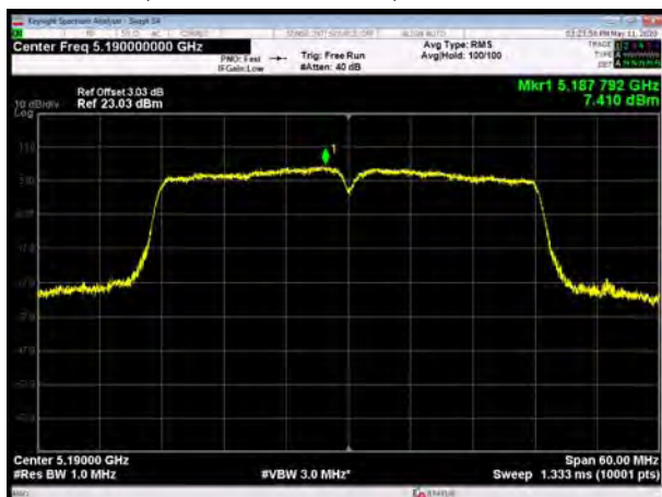
U-NII-1, 802.11ac VHT40, Channel No.: 38
