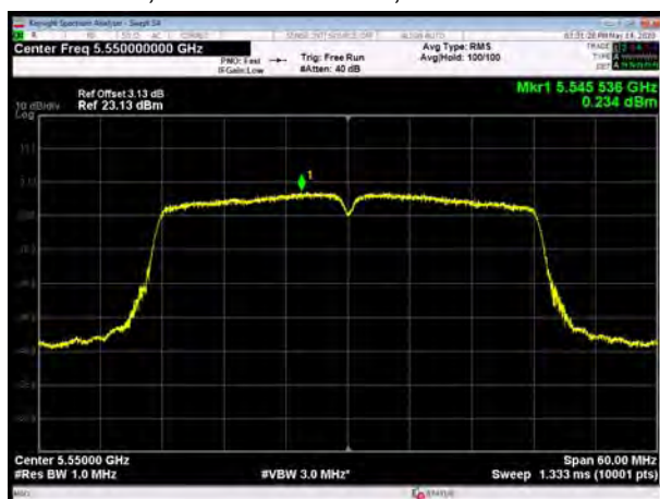
U-NII-2C, 802.11ac VHT40, Channel No.: 110
