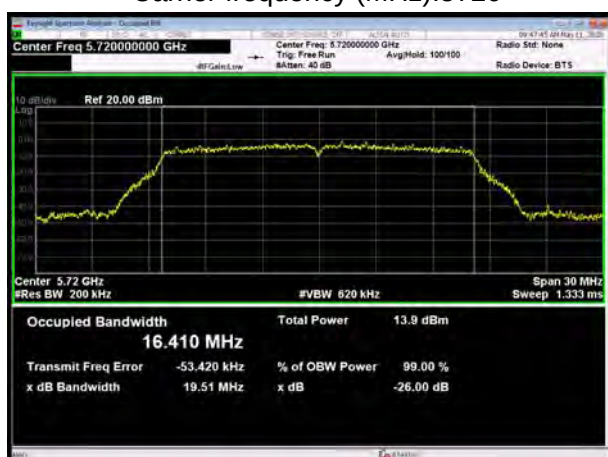
U-NII-2C, 802.11a Carrier frequency (MHz): 5720
