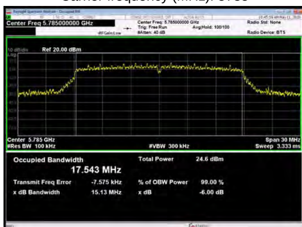
U-NII-3, 802.11ac VHT20 Carrier frequency (MHz): 5785
