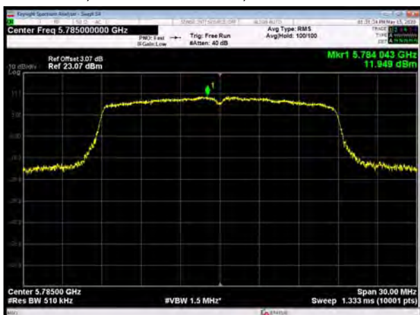
U-NII-3, 802.11ac VHT20, Channel No.: 165
