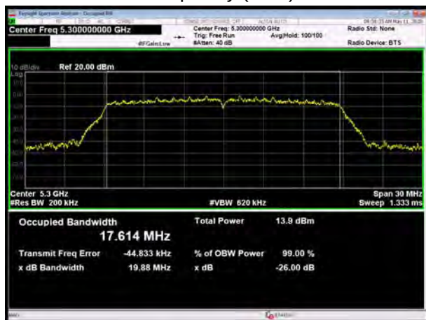
U-NII-2A, 802.11ac VHT20 Carrier frequency (MHz): 5300
