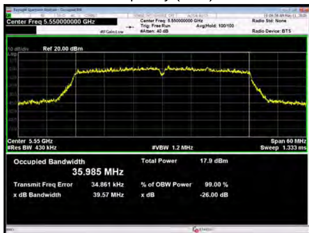
U-NII-2C, 802.11ac VHT40 Carrier frequency (MHz): 5550
