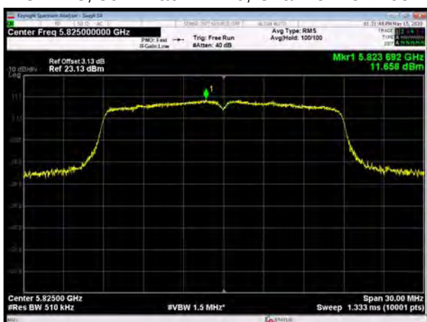
U-NII-3, 802.11ac VHT80, Channel No.: 155
