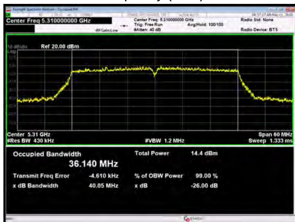
U-NII-2A, 802.11n HT40 Carrier frequency (MHz): 5310
