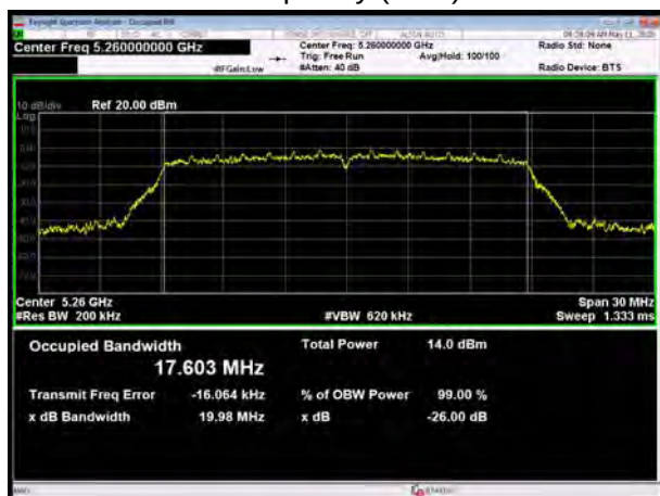
U-NII-2A, 802.11ac VHT20 Carrier frequency (MHz): 5300
