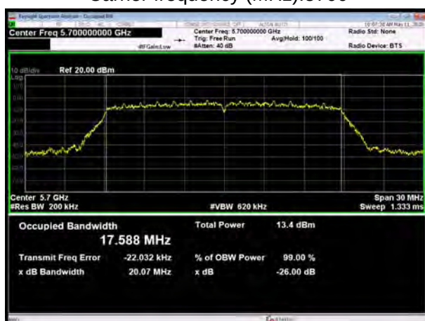
U-NII-2C, 802.11ac VHT20 Carrier frequency (MHz): 5700
