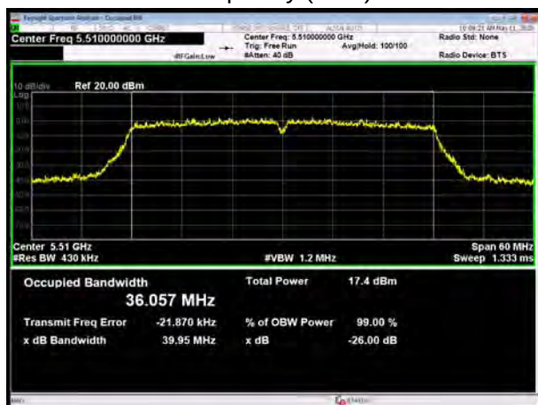
U-NII-2C, 802.11ac VHT40 Carrier frequency (MHz): 5550
