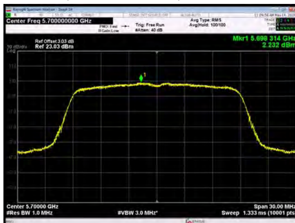
U-NII-2C, 802.11ac VHT20, Channel No.: 140
