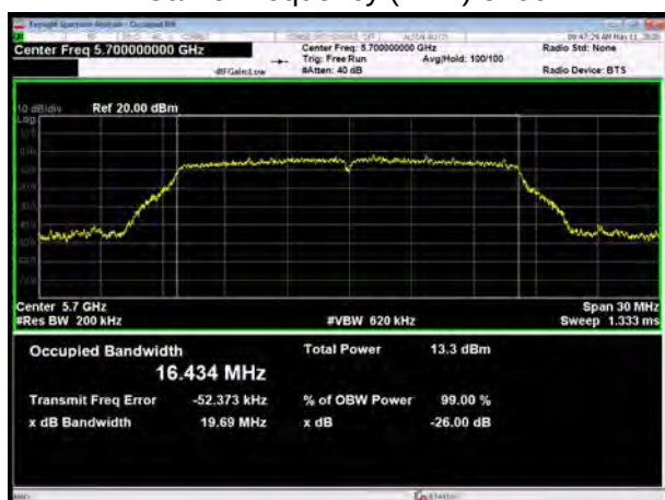
U-NII-2C, 802.11a Carrier frequency (MHz): 5720
