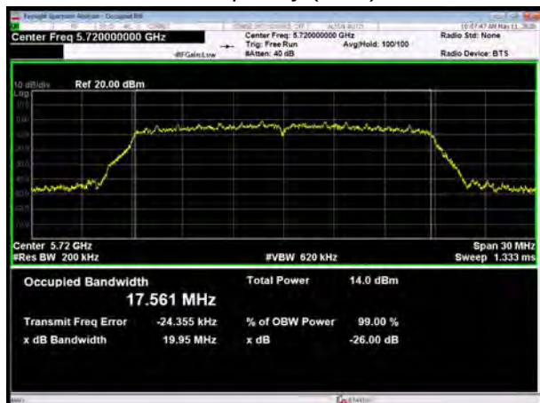
U-NII-2C, 802.11ac VHT20 Carrier frequency (MHz): 5720
