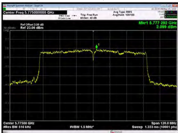
U-NII-3, 802.11ac VHT80, Channel No.: 155
