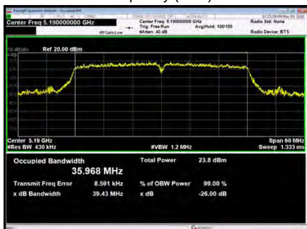
U-NII-1, 802.11ac VHT40 Carrier frequency (MHz): 5190
