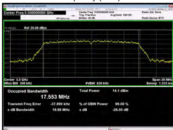
U-NII-2C, 802.11ac VHT20 Carrier frequency (MHz): 5580
