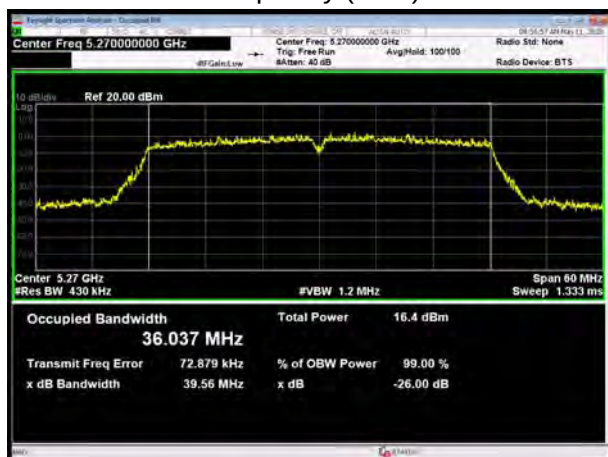
U-NII-2A, 802.11n HT40 Carrier frequency (MHz): 5310
