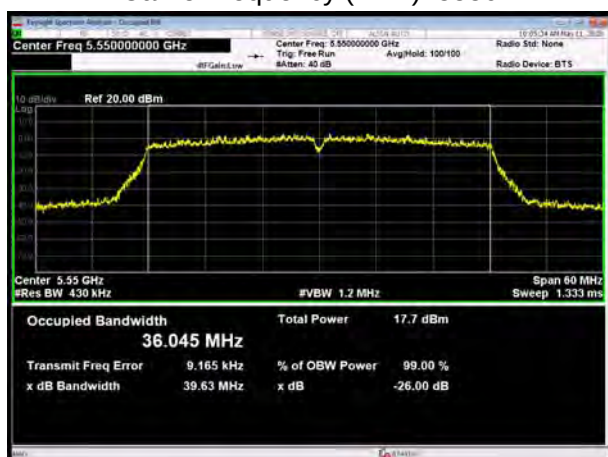
U-NII-2C, 802.11n HT40 Carrier frequency (MHz): 5670
