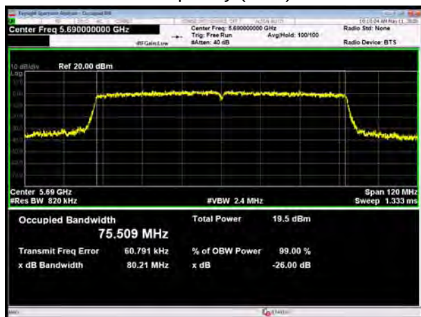
U-NII-2C, 802.11ac VHT80 Carrier frequency (MHz): 5690
