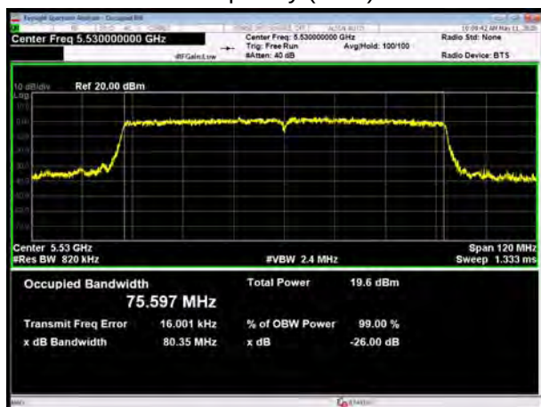
U-NII-2C, 802.11ac VHT80 Carrier frequency (MHz): 5690
