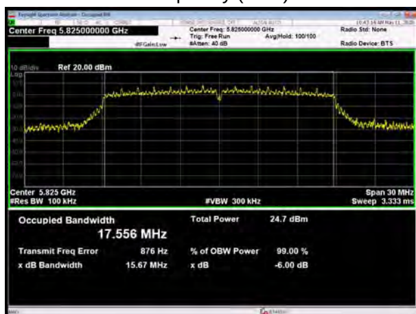
U-NII-3, 802.11ac VHT20 Carrier frequency (MHz): 5745
