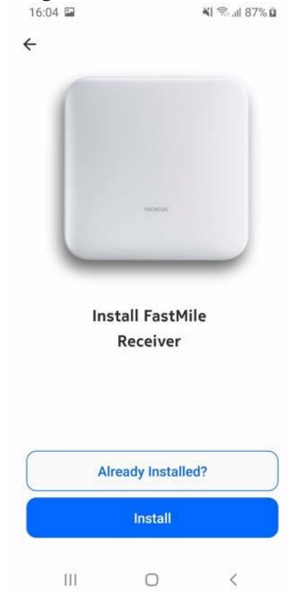
Figure 40 Screen showing the Already Installed option for unit managed by an ACS through TR-069
