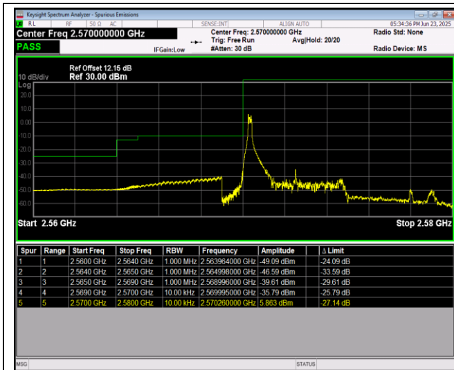
Band38-5MHz-64QAM-37775-25RB#0
