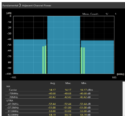
70MHz_30kHz_3585MHz-OFDM QPSK_RB180@0 -40.58,-42.23dB
