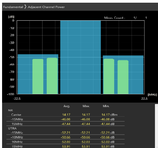
15MHz_30kHz_3557.5MHz-OFDM QPSK_RB36@0 -46.8,-47.16dB
