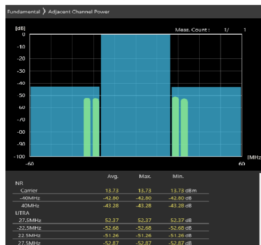
40MHz_30kHz_3680MHz-OFDM QPSK_RB100@0 -42.58,-43.68dB
