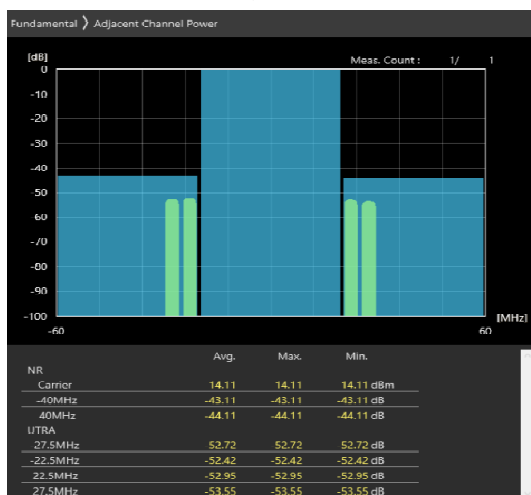
40MHz_30kHz_3680MHz-OFDM QPSK_RB50@25 -43.45,-44.64dB
