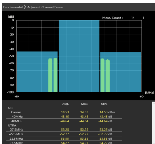
40MHz_30kHz_3680MHz-OFDM QPSK_RB50@25 -43.45,-44.64dB
