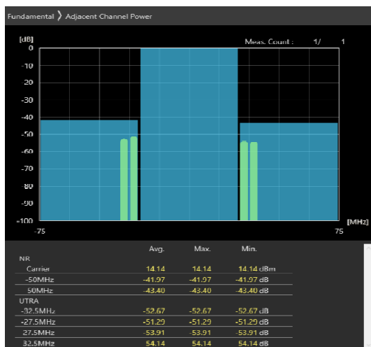
50MHz_30kHz_3575MHz-OFDM QPSK_RB128@0 -41.95,-43.17dB
