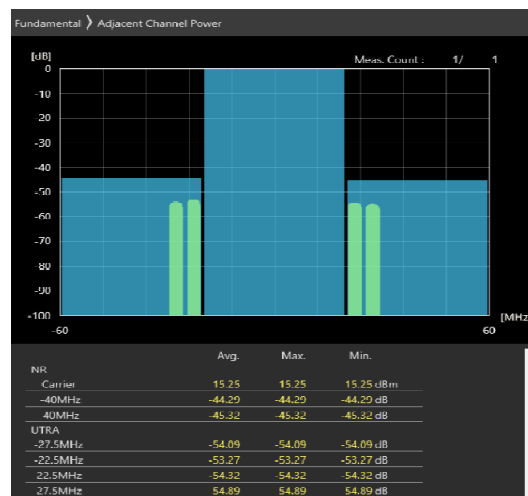
40MHz_30kHz_3680MHz-OFDM QPSK_RB1@105 -42.8,-43.28dB
