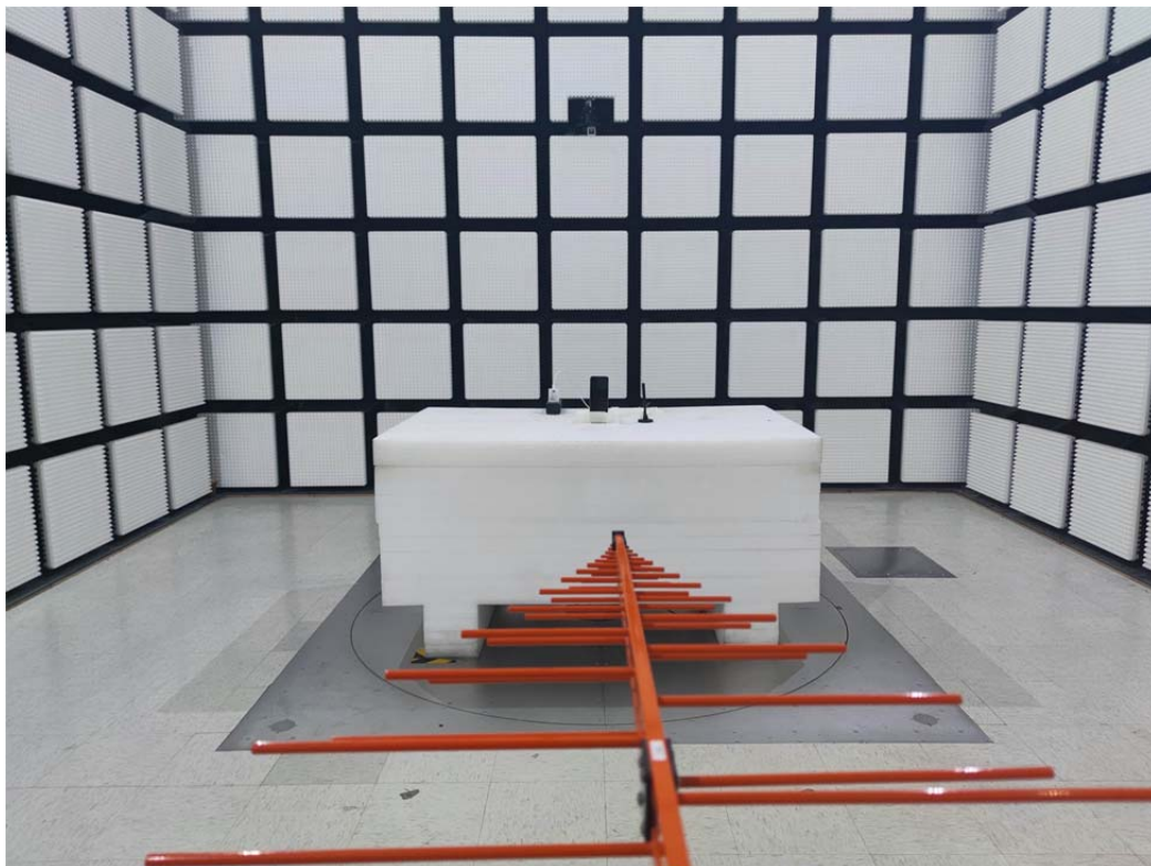
Radiated Emission 30 MHz-1 GHz View
