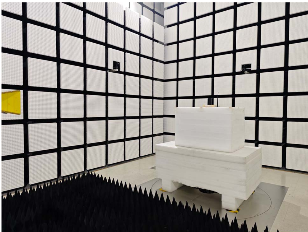
Radiated Emission 1-18GHz View
