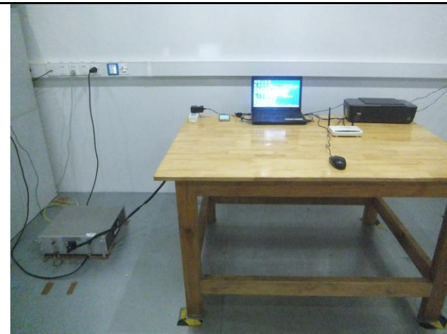
Conducted Emissions Test Setup – Front View
