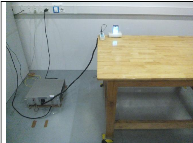
Conducted Emissions Test Setup Front View
