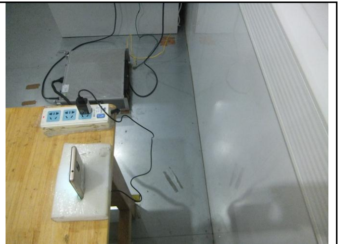
Conducted Emissions Test Setup Side View
