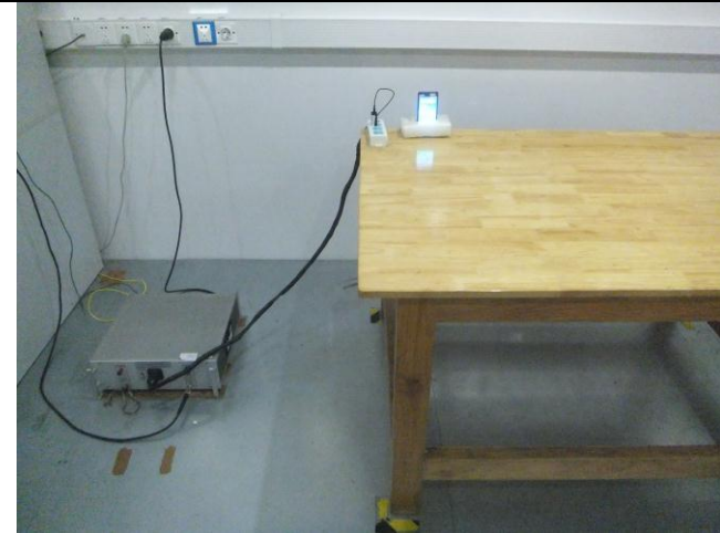
Conducted Emissions Test Setup Front View
