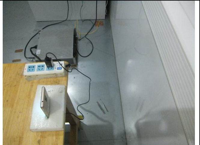
Conducted Emissions Test Setup Side View
