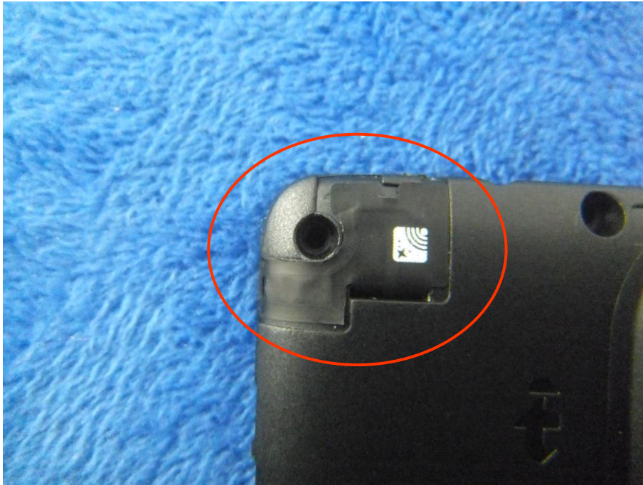
BT - Antenna View
