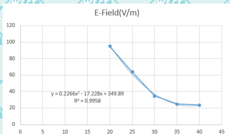
Validate the fitted curve according to KDB 680106, the error between the two nearest test points must not exceed 30%.
