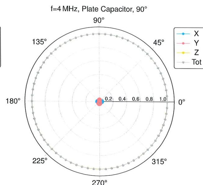
**E-Field Receiving Pattern ( $\phi$ ),  $\vartheta = 0^\circ$**
