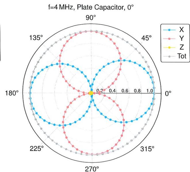
**E-Field Receiving Pattern ( $\phi$ ),  $\vartheta = 90^\circ$**
