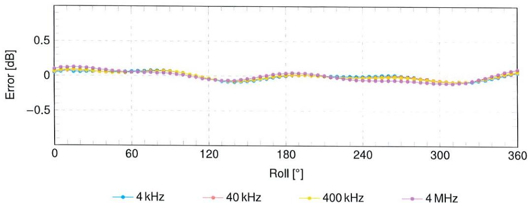
**E-Field Receiving Pattern ( $\phi$ ),  $\vartheta = 90^\circ$**
