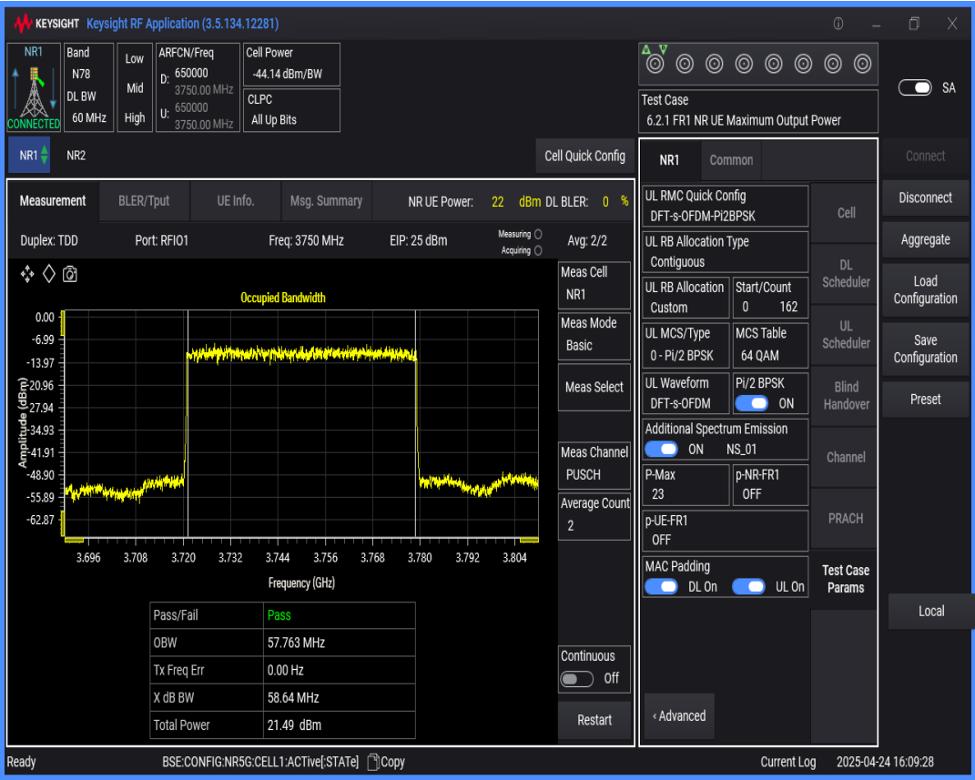
n78(3700-3800) SCS=30kHz DFT_BPSK BW=90MHz Channel=650000 RB=240@0
