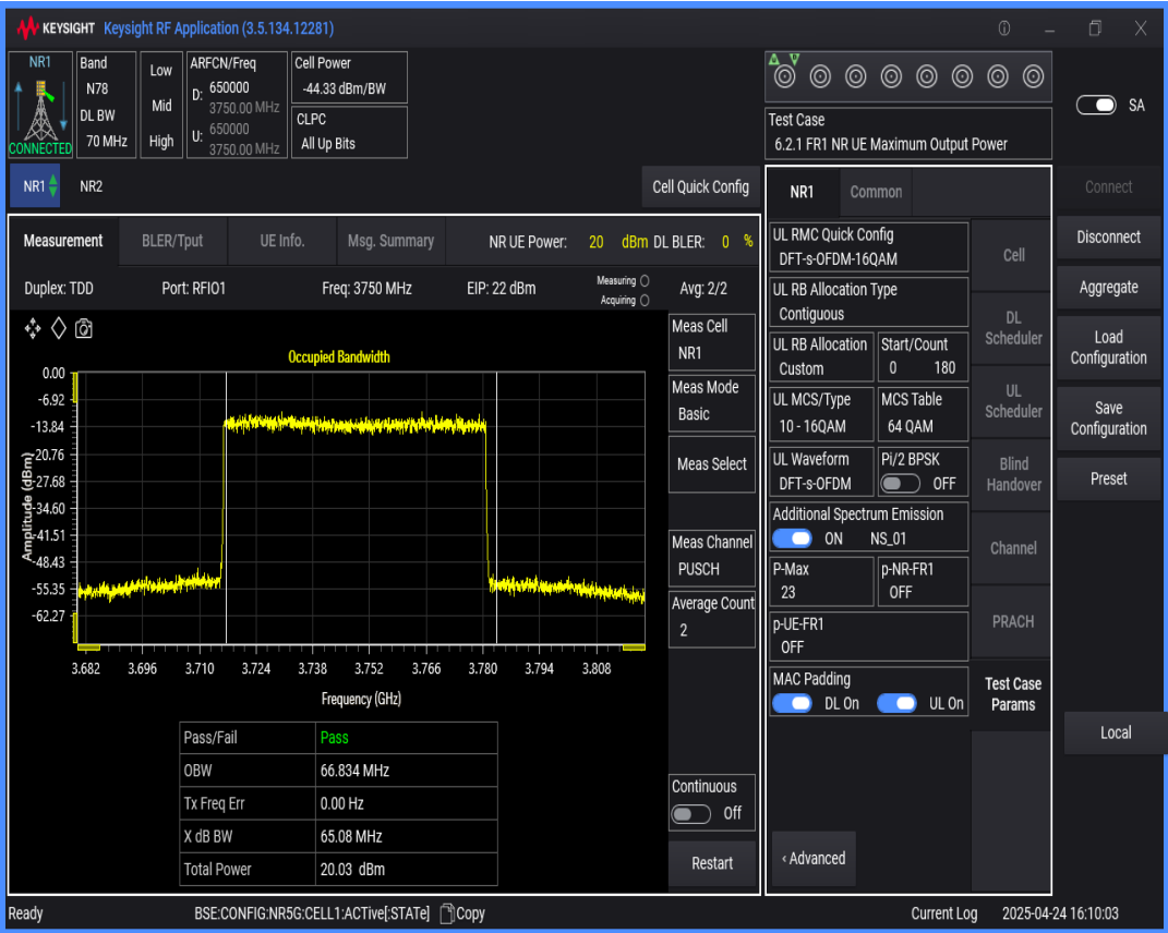
n78(3700-3800) SCS=30kHz DFT_QAM256 BW=100MHz Channel=650000 RB=270@0
