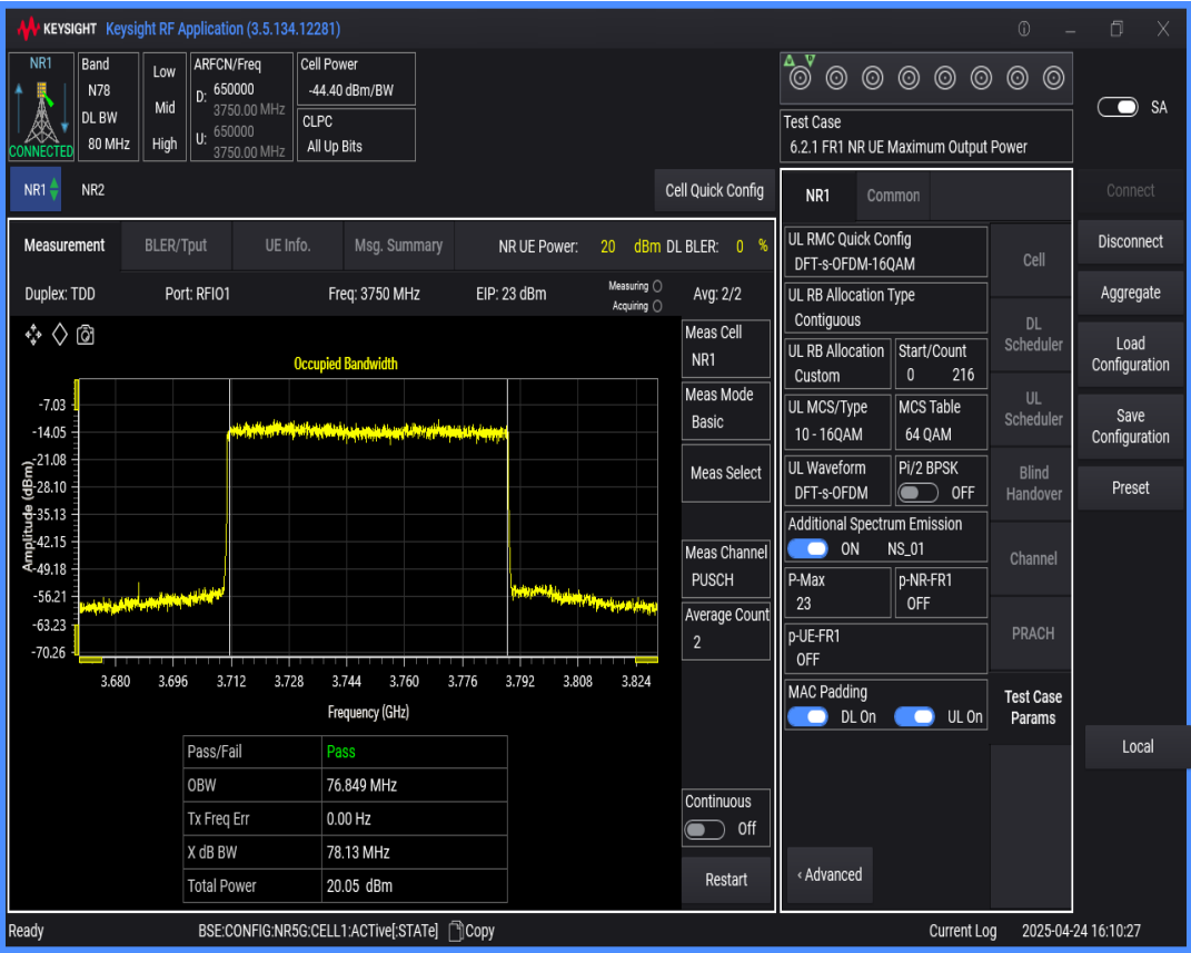
n78(3700-3800) SCS=30kHz DFT_QAM256 BW=10MHz Channel=650000 RB=24@0
