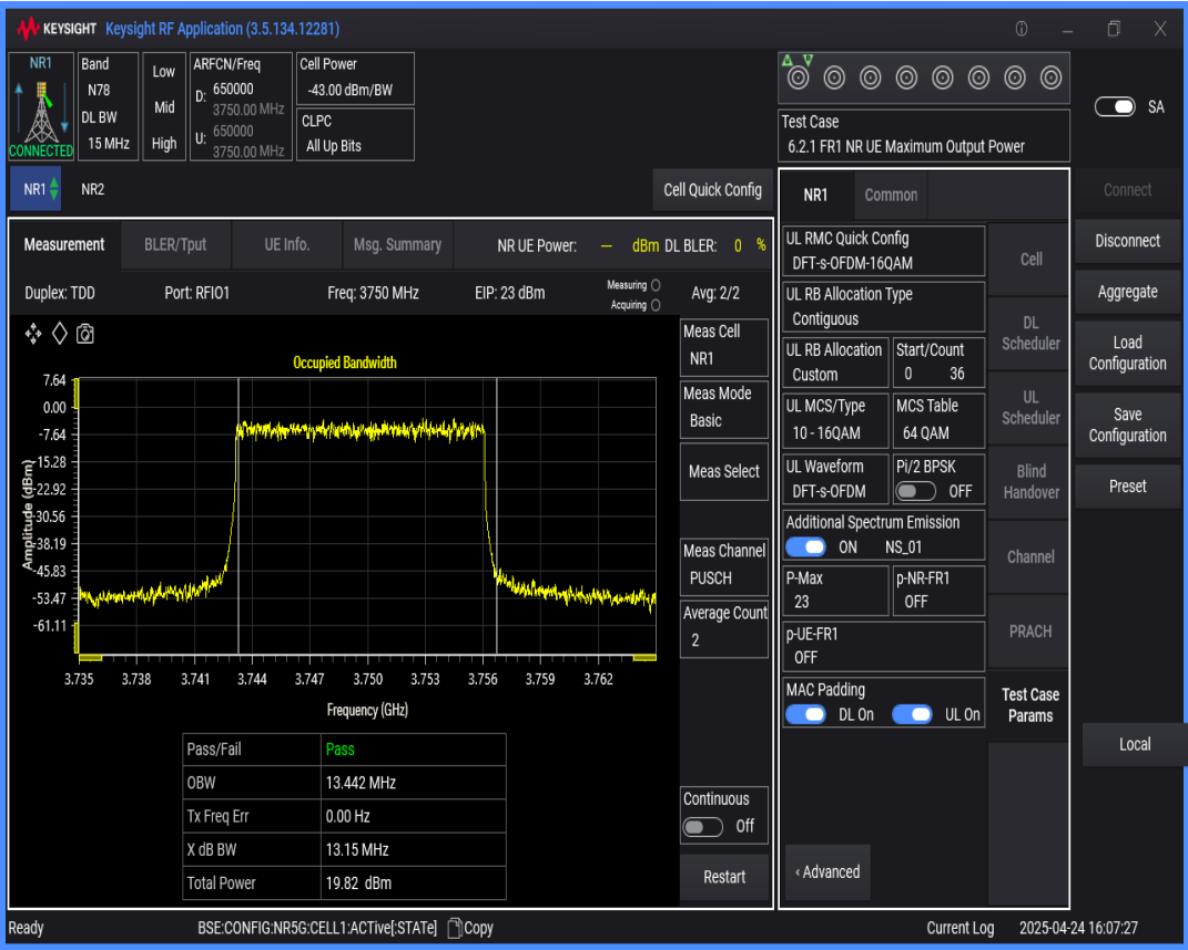
n78(3700-3800) SCS=30kHz DFT_QAM16 BW=50MHz Channel=650000 RB=128@0
