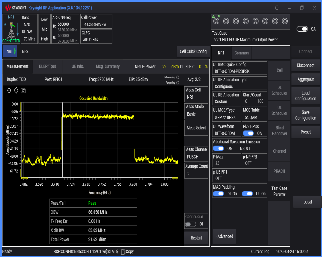
n78(3700-3800) SCS=30kHz DFT_BPSK BW=60MHz Channel=650000 RB=162@0
