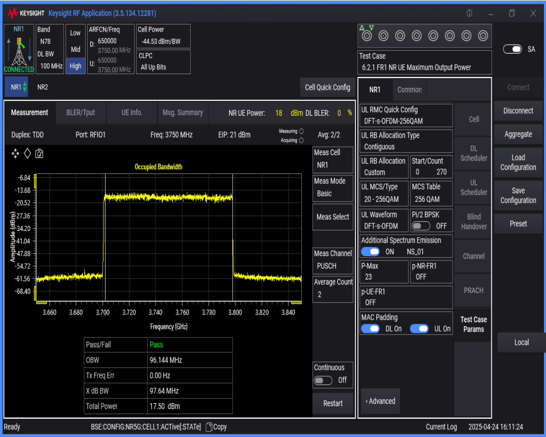
n78(3700-3800) SCS=30kHz DFT_QAM16 BW=90MHz Channel=650000 RB=240@0
