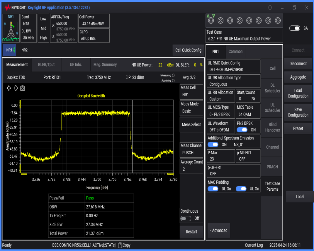
n78(3700-3800) SCS=30kHz DFT_BPSK BW=70MHz Channel=650000 RB=180@0
