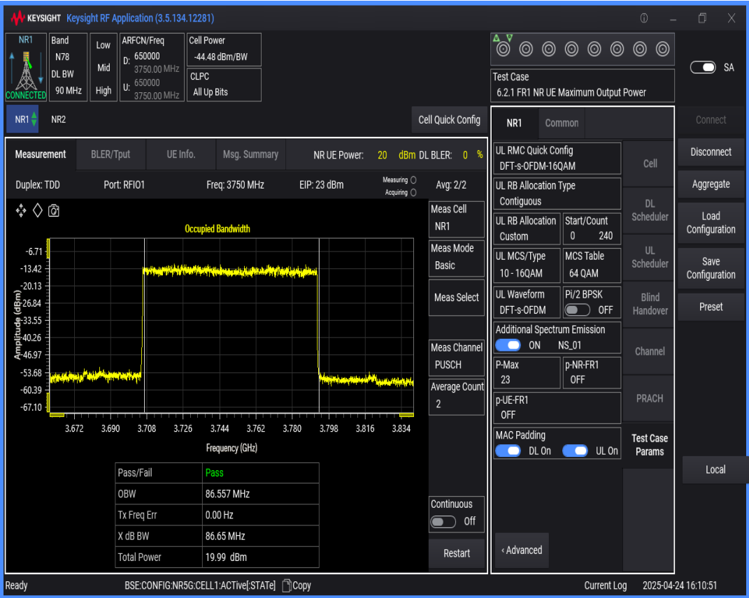
n78(3700-3800) SCS=30kHz DFT_QAM16 BW=80MHz Channel=650000 RB=216@0
