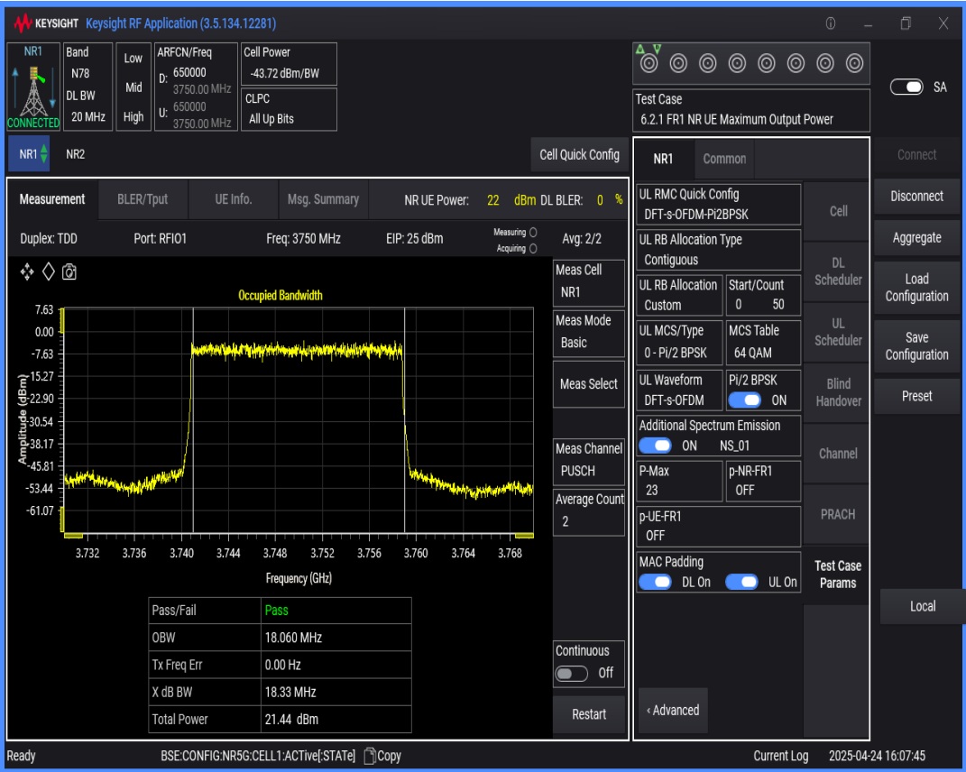
n78(3700-3800) SCS=30kHz DFT_BPSK BW=50MHz Channel=650000 RB=128@0
