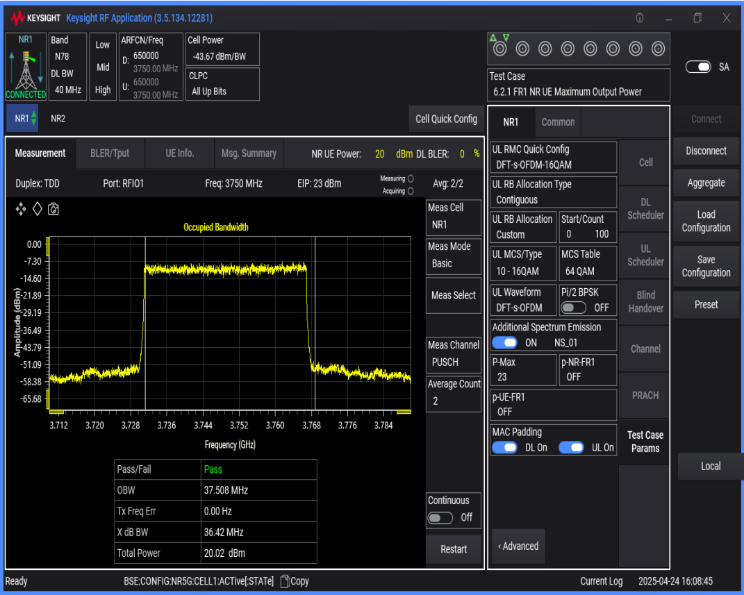
n78(3700-3800) SCS=30kHz DFT_QAM16 BW=30MHz Channel=650000 RB=75@0
