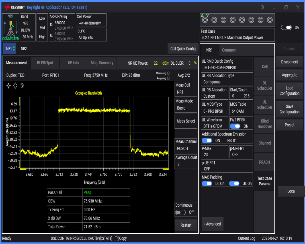
n78(3700-3800) SCS=30kHz DFT_QAM16 BW=100MHz Channel=650000 RB=270@0
