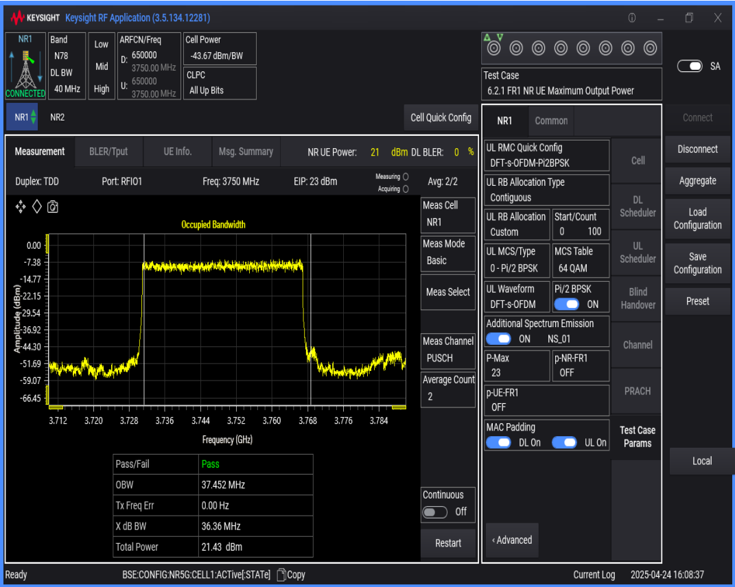
n78(3700-3800) SCS=30kHz DFT_BPSK BW=30MHz Channel=650000 RB=75@0
