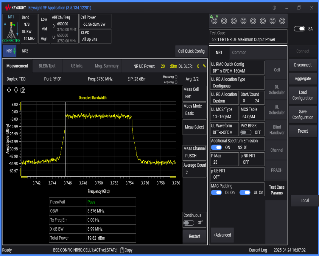
n78(3700-3800) SCS=30kHz DFT_QAM16 BW=20MHz Channel=650000 RB=50@0
