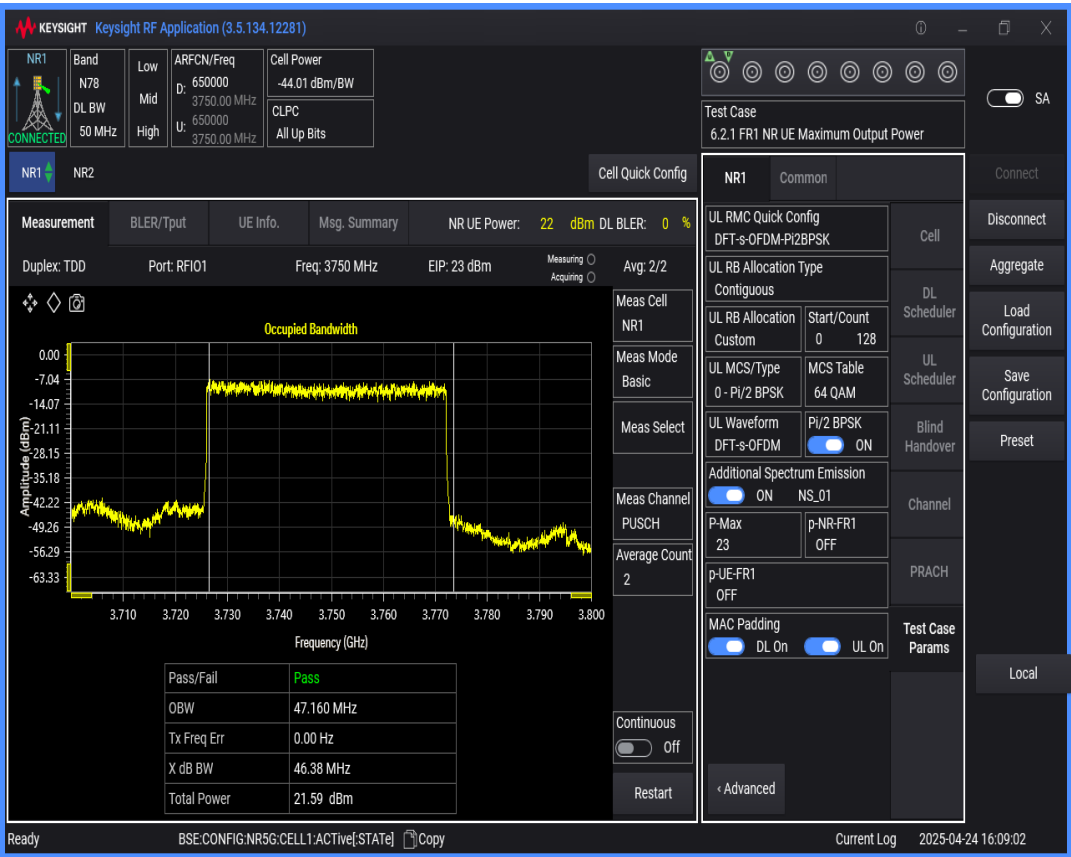
n78(3700-3800) SCS=30kHz DFT_BPSK BW=40MHz Channel=650000 RB=100@0
