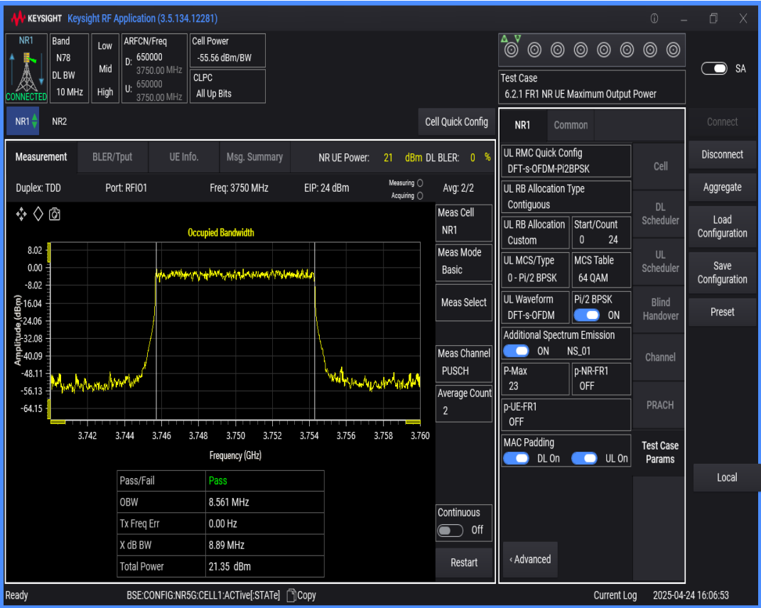
n78(3700-3800) SCS=30kHz DFT_BPSK BW=15MHz Channel=650000 RB=36@0
