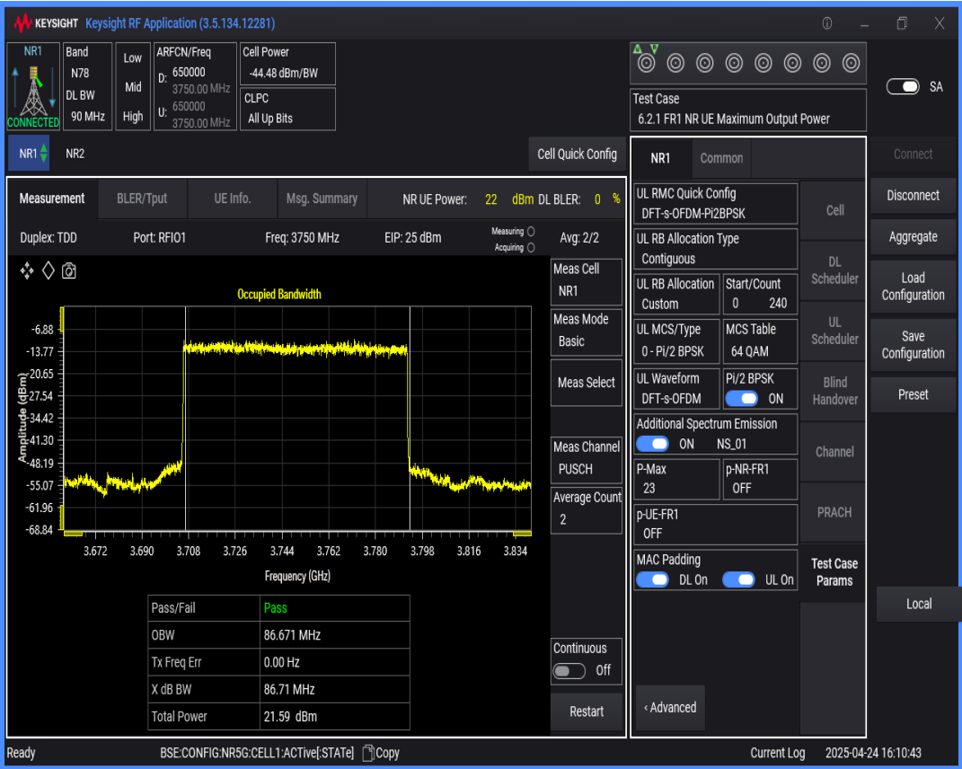
n78(3700-3800) SCS=30kHz DFT_BPSK BW=80MHz Channel=650000 RB=216@0
