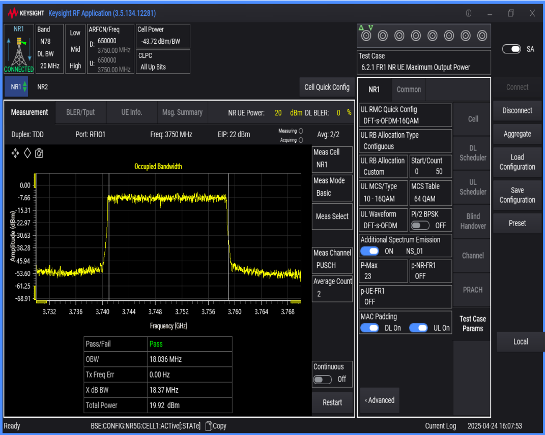
n78(3700-3800) SCS=30kHz DFT_QAM16 BW=15MHz Channel=650000 RB=36@0
