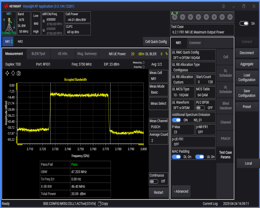
n78(3700-3800) SCS=30kHz DFT_QAM16 BW=40MHz Channel=650000 RB=100@0
