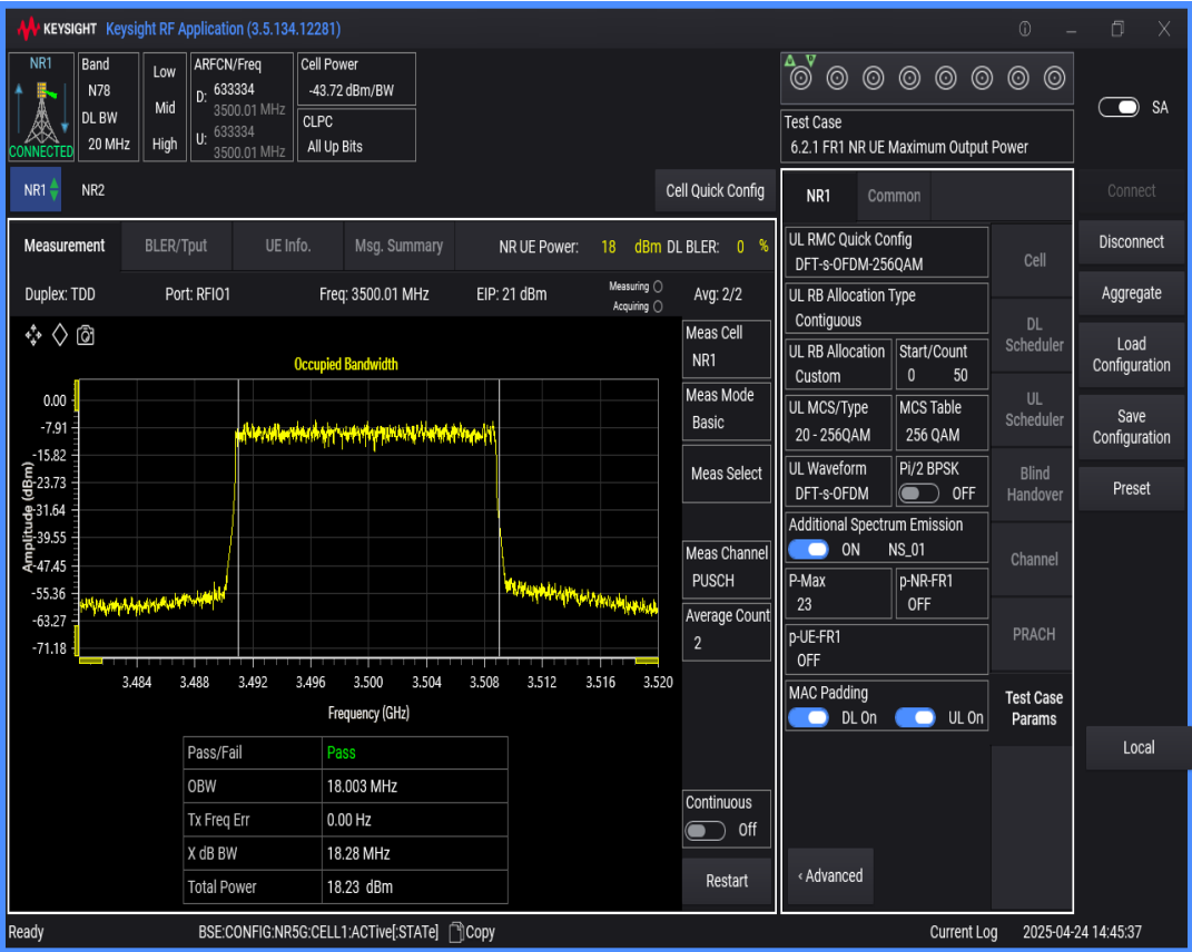
n78(3450-3550) SCS=30kHz DFT_QAM256 BW=40MHz Channel=633334 RB=100@0
